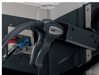
Figure 1: Picture of the Antaris Fiber Port and SabIR reflectance probe
