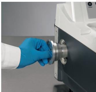
Figure 1. Changing the source assembly on a Thermo Scientific Antaris FT-NIR analyzer
