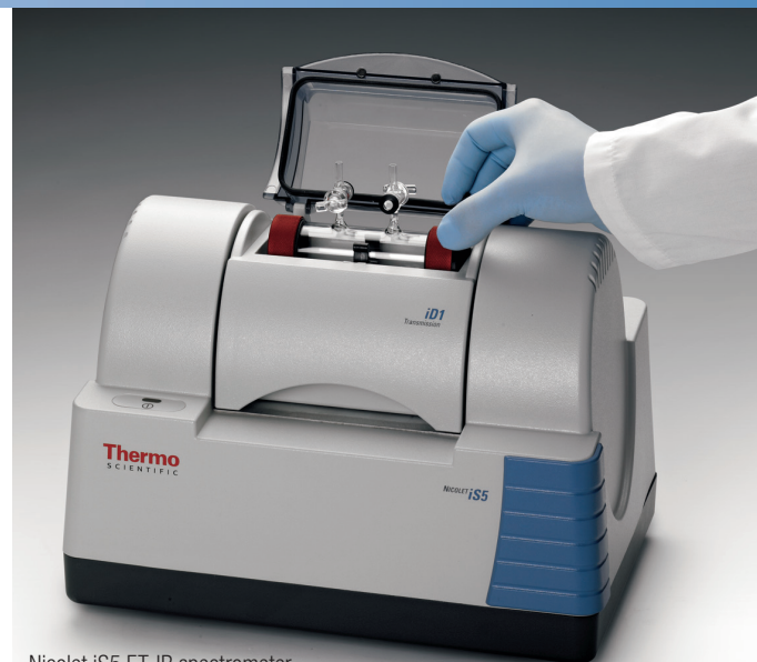
Nicolet iS5 FT-IR spectrometer with 10 cm gas cell
