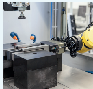
Sample loading and unloading by the ARL SMS-2500 system robot
