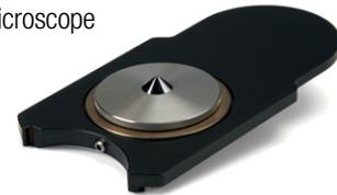
This ATR's germanium crystal is multi-coated to guarantee a minimum throughput of 50% and it has a robust design to allow surveys while in contact with the sample, as well as a practical slide mount for ease of cleaning. The precise and robust mechanism guarantees perfect repositioning of the crystal. The 350  $\mu\text{m}$  diameter micro tip offers a perfect balance between small contact area and high durability.
