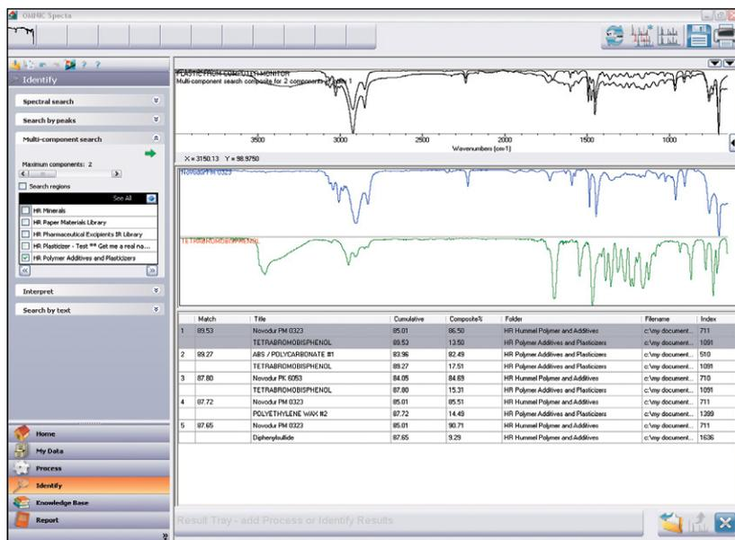
OMNIC Specta provides innovative identification and interpretation tools and an unique expert knowledge base. It converts all of the data on your hard disk into an always-ready database and includes a standard collection of 9000 spectra that enables you to efficiently and effectively identify materials. And when even the microscope spatial resolution reaches its limits, OMNIC Specta adds the power of identifying mixed compounds with a mouse click.
