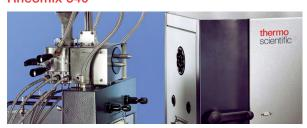
The internal mixer Thermo Scientific HAAKE Rheomix 540 is specially designed for testing the behavior of thermosetting compounds with respect to flow and rate of cure.
