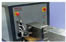
Because of its conical design, the Twin Screw Compounder Thermo Scientific HAAKE Rheomex CTW100 realizes very short dwell times and avoids dead volume. This leads to its strength in the following typical applications:
