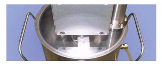
The Thermo Scientific HAAKE PlanetMix 500 OS planetary mixer with the planetary rotor is designed for mixing and testing of solid powders with liquids.
