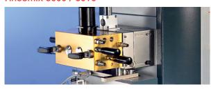
The Thermo Scientific HAAKE Rheomix 3000 enables production of small batches simultaneous recording of torque and mass temperature (due to its larger chamber volume). Due to its high torque capability, it is ideal for applications in the rubber industry, such as testing of the melting and scorch behavior of rubber compounds. The mixing chamber is electrically heated and air-cooled, and the front and back plates are electrically heated as well.
