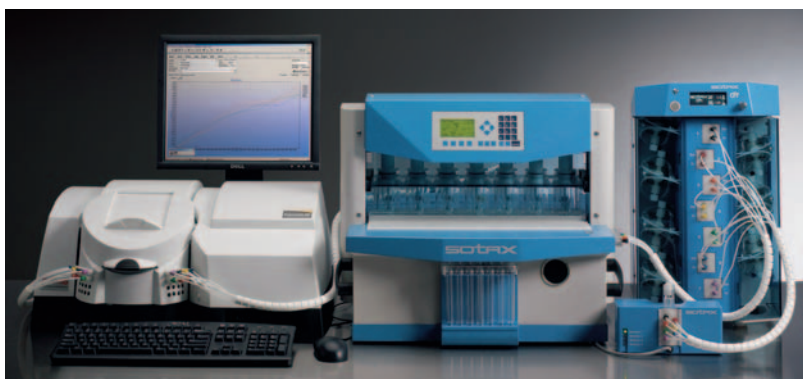
Evolution 300 with the SOTAX Apparatus IV flow-through system offers a unique solution for a variety of Tablet Dissolution assays
