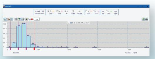
Distribution histogram of AI single spark intensities in a low alloy steel sample.
