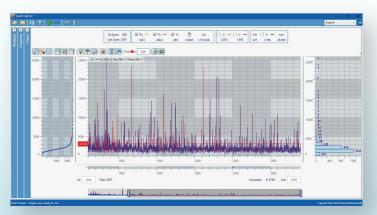
Display of S-chart, run chart and histogram of Al single spark signals in a low alloy steel sample.
