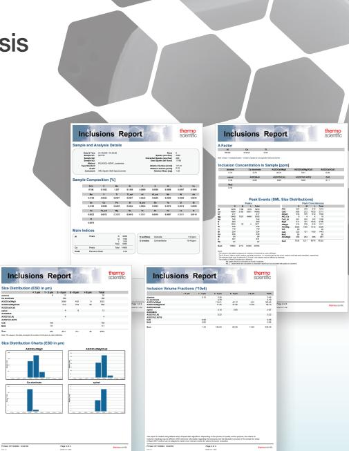
Example of an inclusion analysis report of a low alloy steel sample measured with Advanced Inclusion Analysis method.
