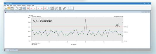
SPC run chart of aluminum oxides in 50 steel production samples. Number of inclusions in sample 30 is above USL, which signifies that its inclusion content is not compliant.
