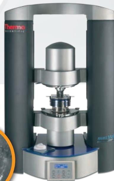
MARS Rheometer platform with RheoScope module
