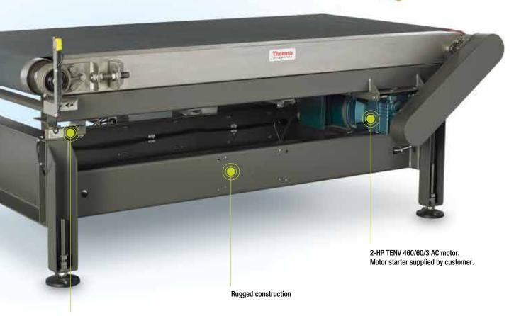
Four-load-cell design allows for high-speed weighing and is virtually indestructible for overloads; rugged construction—
