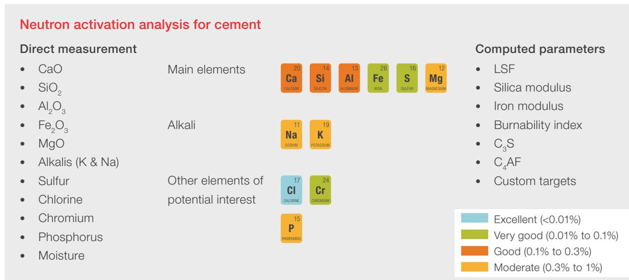
Figure 2: PGNAA and PFTNA capabilities in cement production
