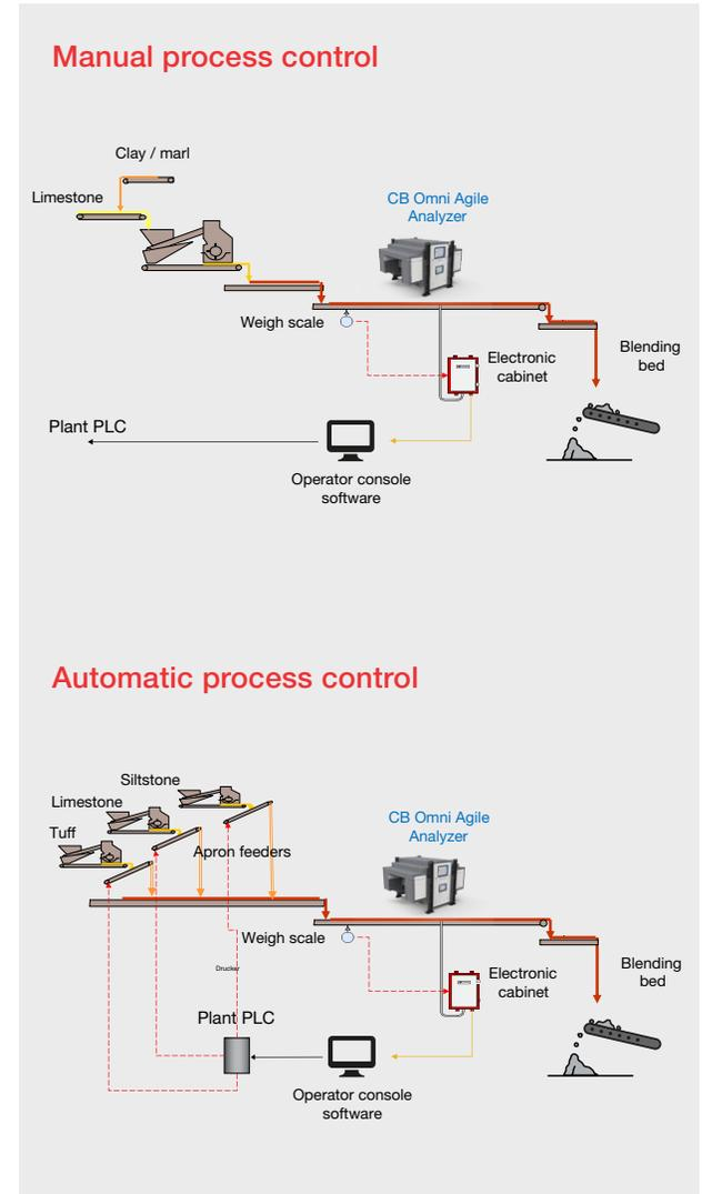
Figure 6: Manual versus automated process control
