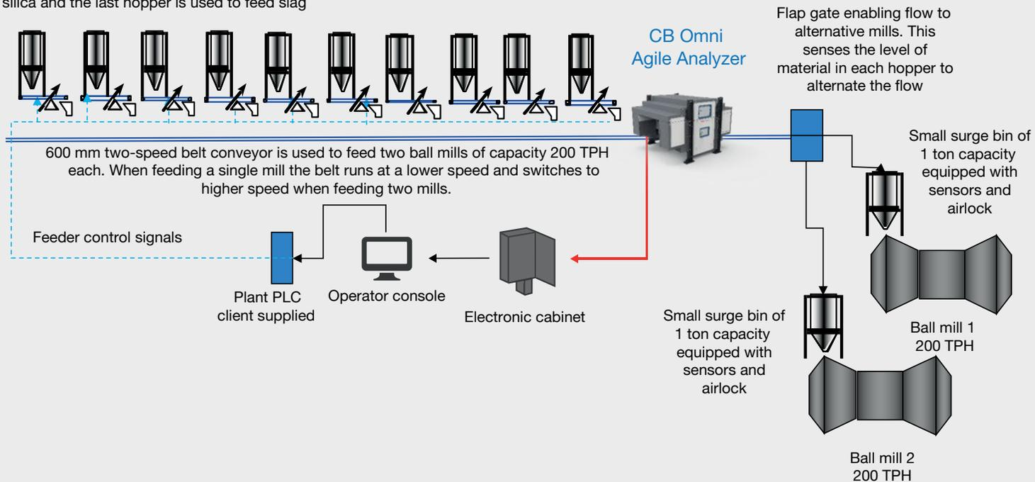
Figure 9: Depiction of an automated, integrated solution that is both efficient and sustainable
