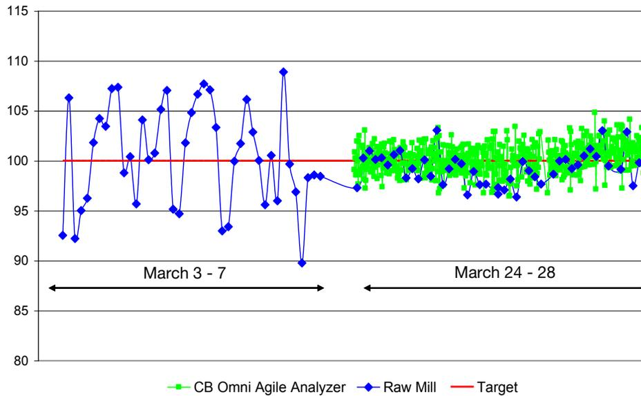
The Thermo Scientific analyzer and RAMOS software have allowed “an improvement in the standard deviation to about half of what it was coming out of the raw mill” compared to prior to installation.
