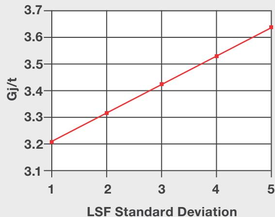
Figure 11 quantifies the impact of LSF variability and shows how much LSF stability is worth in terms of fuel savings. These savings alone deliver an attractive ROI on the implementation of real-time elemental analysis and are typically sufficient to justify an investment.
