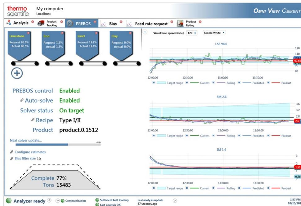
Figure 7: PREBOS software managing feed rate for four different materials
