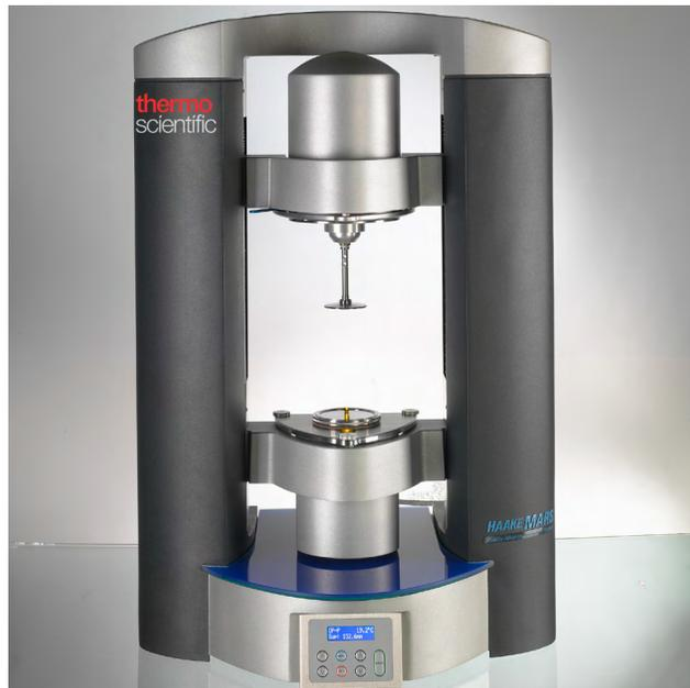
HAAKE MARS com o módulo RheoScope
