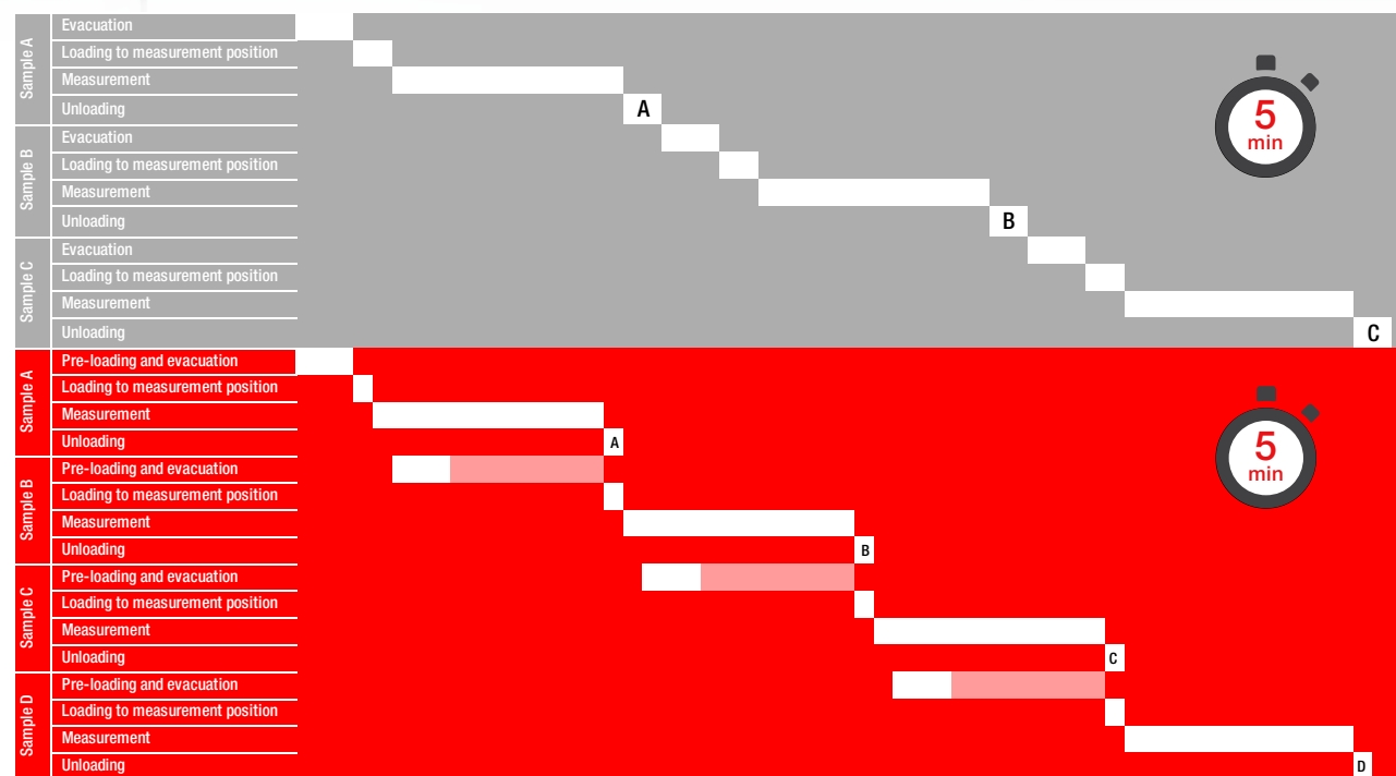
Sequencing of sample loading: single-sample loader (top, grey) vs. ARL X900 dual-sample loader (bottom, red). Time estimated for analyzing four metallic samples with 60-second measurements.
