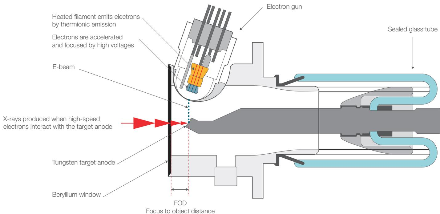
Figure 1. Layout diagram of a microfocus x-ray tube.
