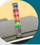
Safety is assured via an LED light pole, multiple e-stops, X-ray key switch, inspection area door lock and safety interlocks on all doors.
