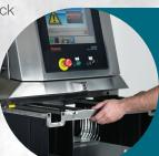
No-lead X-ray shielding curtains on fully adjustable and removable frame for safety, flexibility and easy maintenance.
