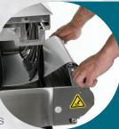
Change a conveyor belt in minutes. Modular design with many infeed/outfeed lengths, rejecters, bins, and shields.
