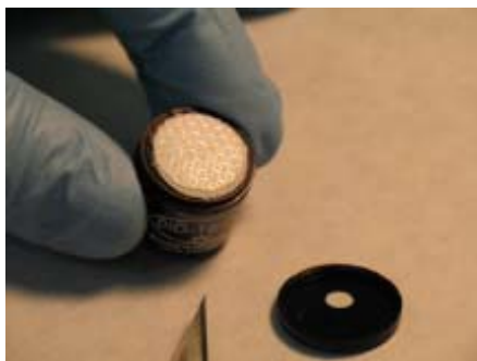
Figure 7-5. Removing the Filter Media
