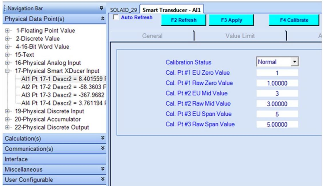
**Figure G-3.** Physical Smart XDucer Input Table
