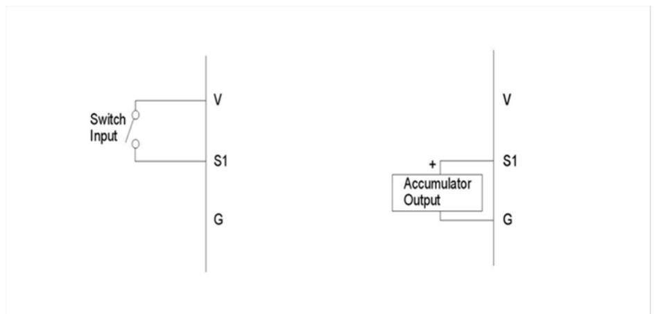
**Figure 3-2.** Digital Input Function
