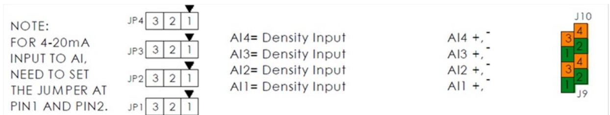
Figure G-2. A1 Test Wiring to J9
