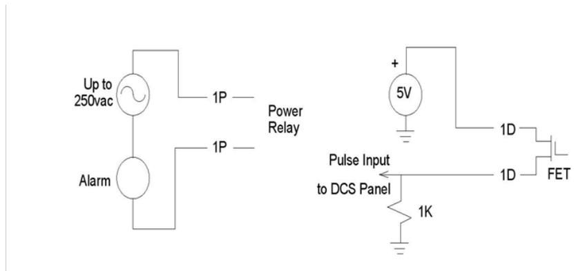
**Figure 3-1.** Digital Output Function
