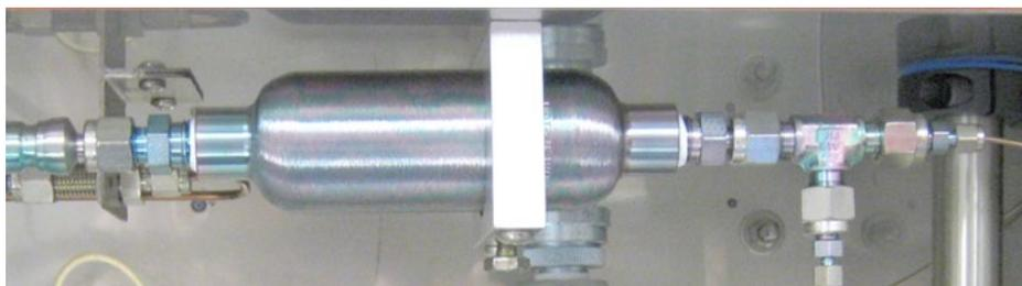
**Figure 2-5.** Typical mixing chamber
