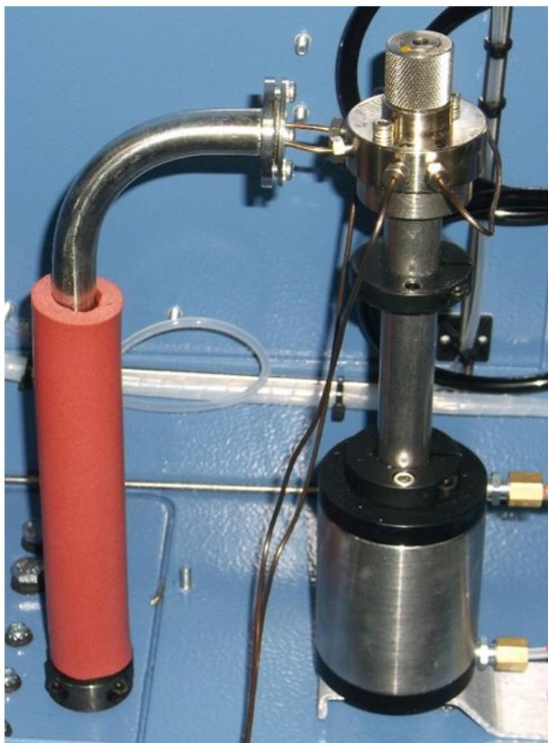
**Figure 2-6.** Uncovered Injection Valve – Liquid Applications
