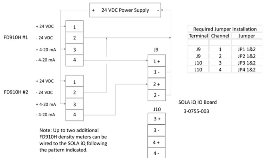
**Figure B-1.** Sarasota FD910H density meter to SOLA iQ connections
