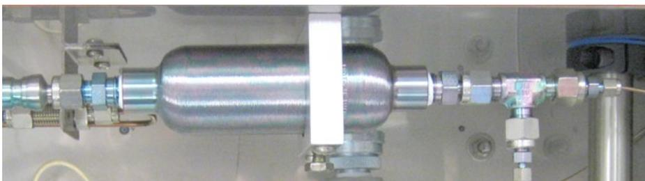
**Figure 2-5.** Typical mixing chamber
