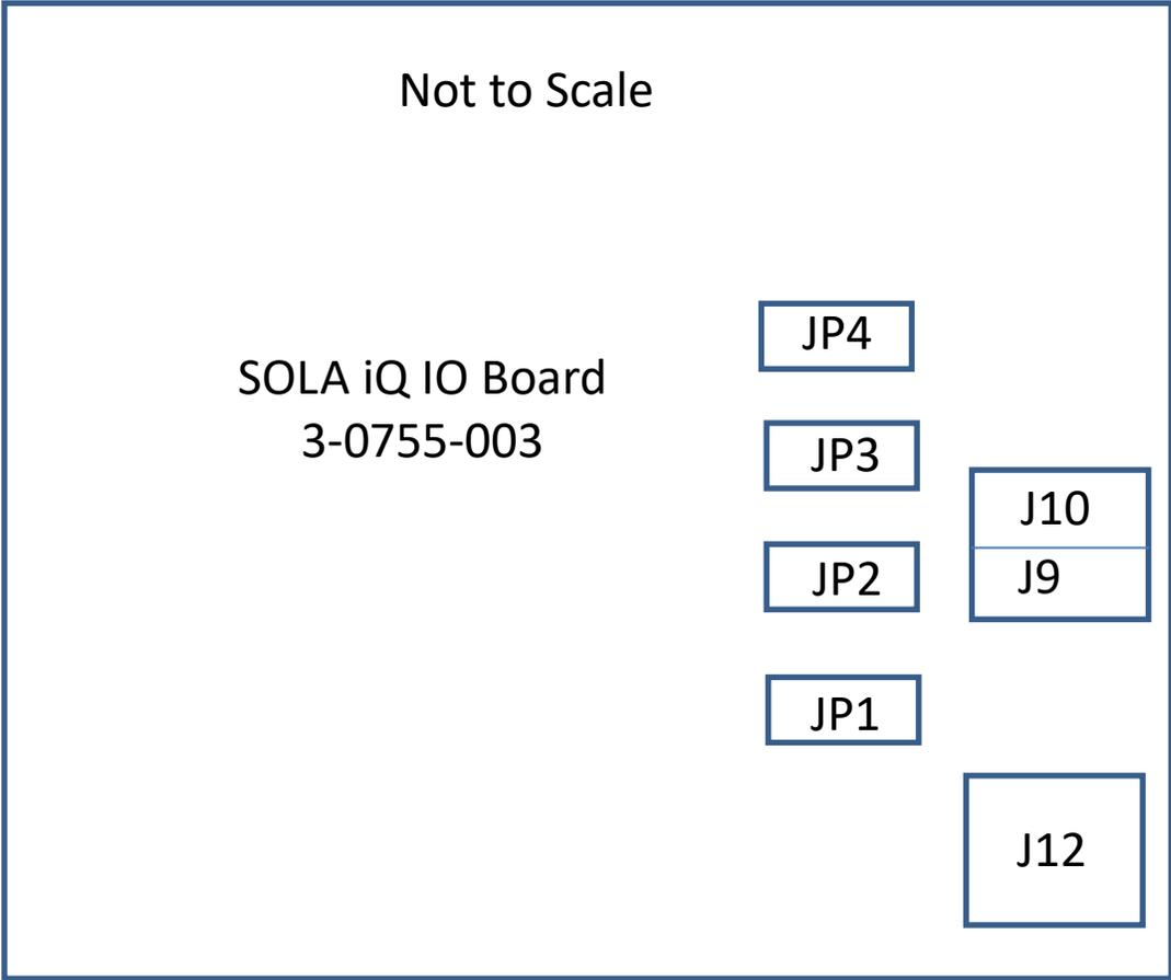
**Figure B-4.** Terminal block connectors on SOLA iQ IO board 3-0755-003
