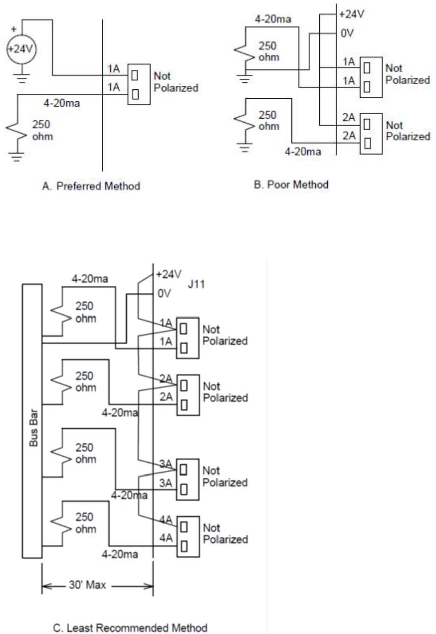
**Figure 3-4.** Analog Output Function
