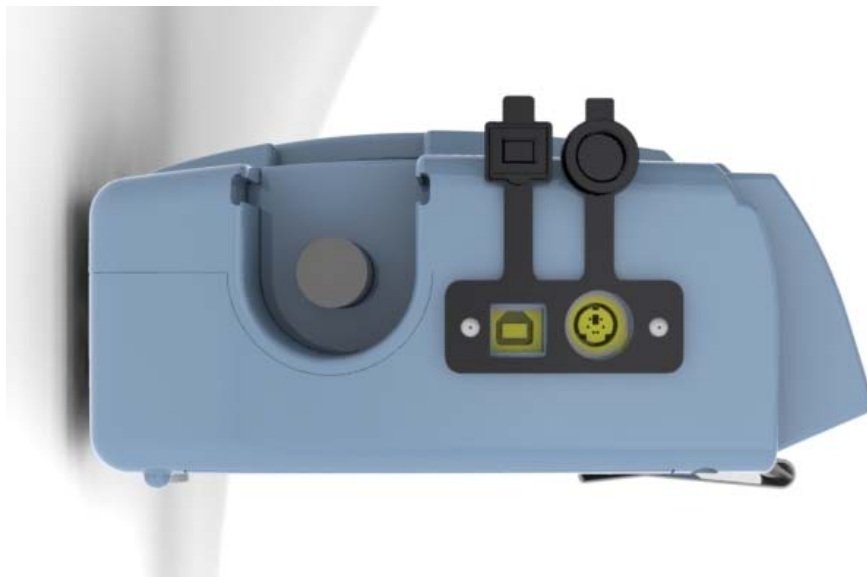
Figure 2–3. Side PM Inlet, USB, RS-232/Analog Panel
