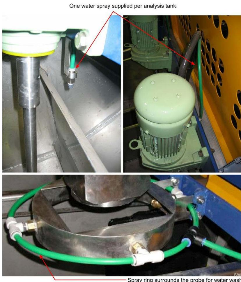
**Figure 5-14.** Water Spray per Analysis Tank and for Probe Washing
