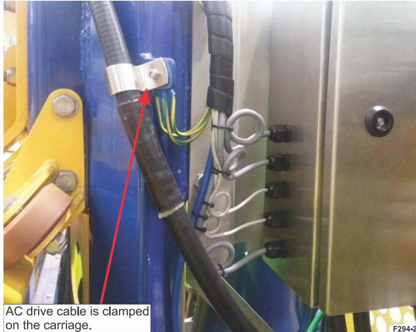
**Figure 5-8.** Attaching the motor conduit to the carriage
