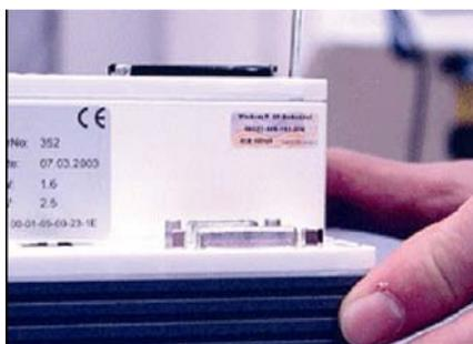
FIG 4-21.1: Ejecting the CF card
