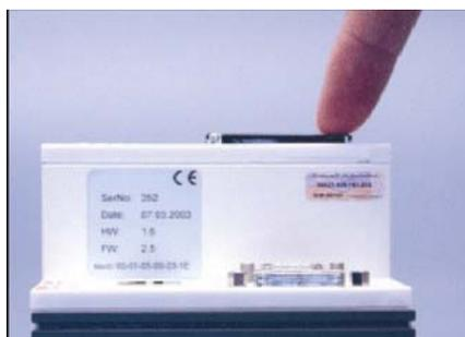
FIG. 4-21.3: Inserting the CF card
