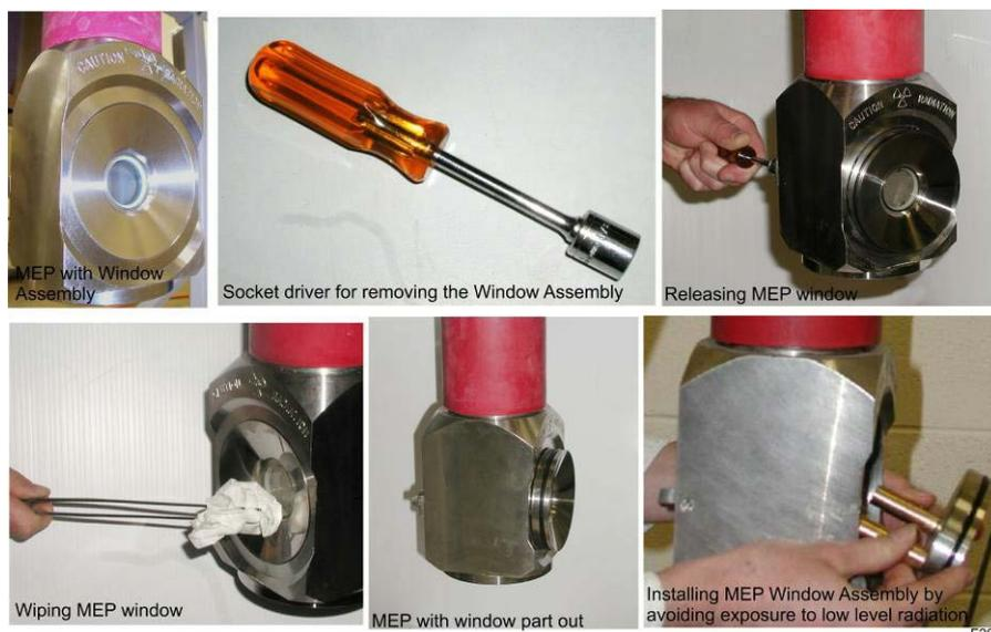
**Figure 8-4.** Cleaning and Replacing the Probe Window
