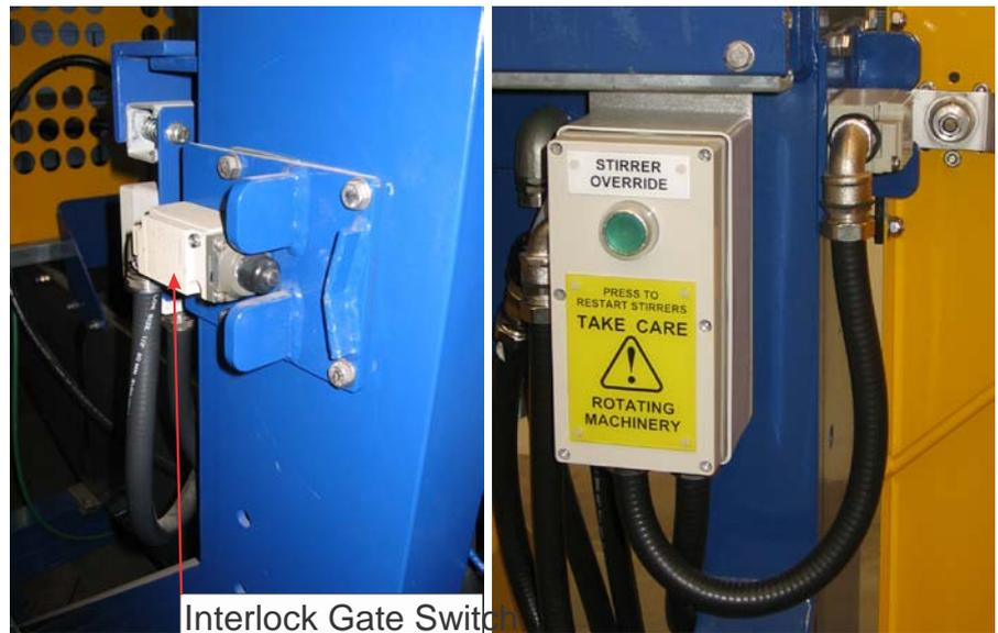
**Figure 7-4.** A door interlock and the Stirrer Override switch
