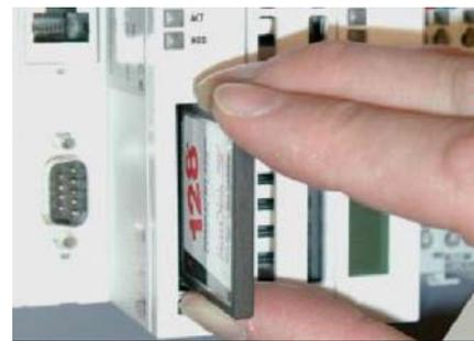
FIG 4-21.2: Removing the CF card
