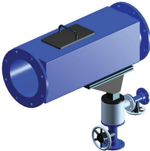
This type of sampler can be used in all gravity flow situations in a pipe or where a pressure pipe sampler cannot be installed. A gravity sampler generally has a 50mm (2") NB sample outlet (flanged) and so a sample delivery pipe line with the same or larger NB size should be used. *These samplers cannot be used for metallurgical accounting purposes.*
