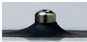
Droplet flattens on unconditioned pedestal
