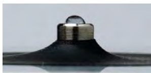
Droplet “beads up” on properly conditioned pedestal
