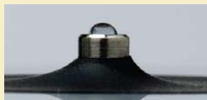
Droplet “beads up” on properly conditioned pedestal
