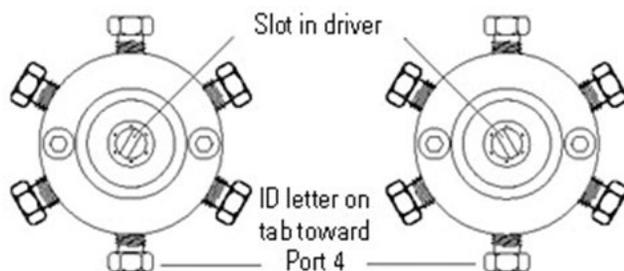
**Figure D-4.** C6 W valve with preload and rotor removed (preload end view)
