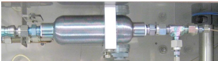
**Figure 8–5.** Mixing Chamber
