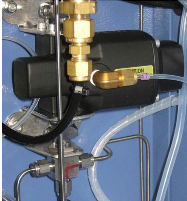
**Figure 4–29.** Sample diverter valves
