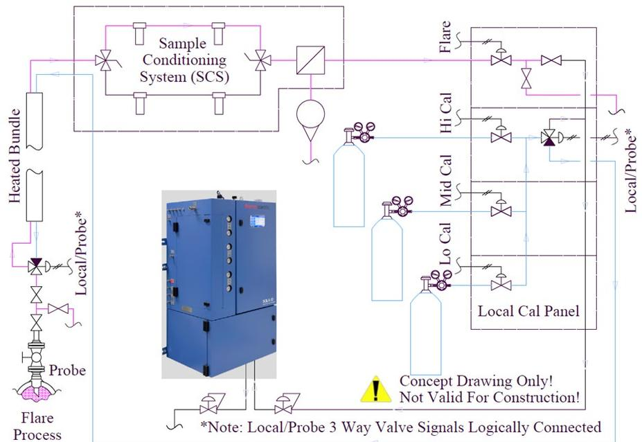
During normal operation, the Probe samples the Flare Process and flows the sample through a heated bundle to the analyzer sample conditioning system. The sample next flows through filters and valves and a forward pressure regulator to the injection valve inside the oven of the SOLA iQ. The sample then flows through the injection valve and out through the back pressure regulator.
