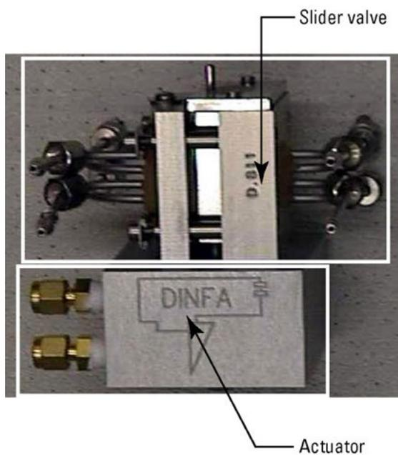
**Figure E-5.** Dinfa 8-port liquid injection valve
