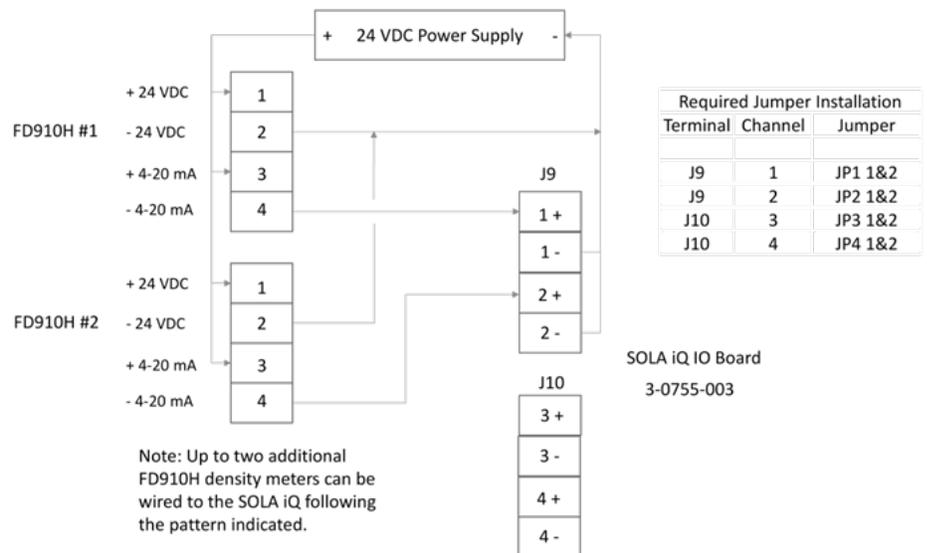
**Figure F-1.** Sarasota FD910H density meter to SOLA iQ connections
