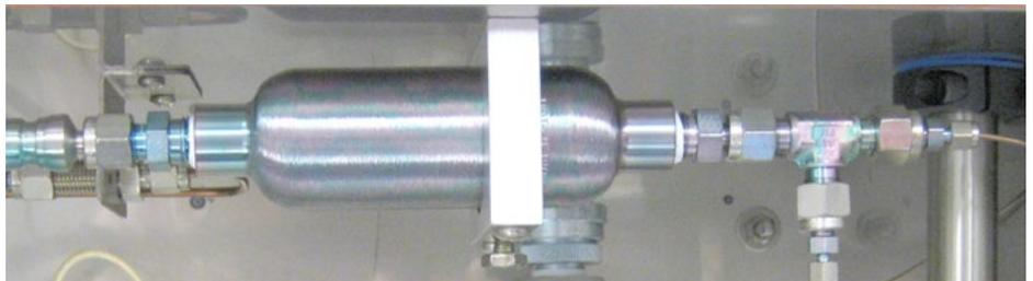
**Figure 2-5.** Typical mixing chamber
