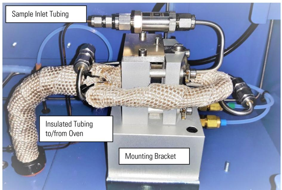
**Figure E-1.** Dinfa Valve mounted in Pneumatics Section
