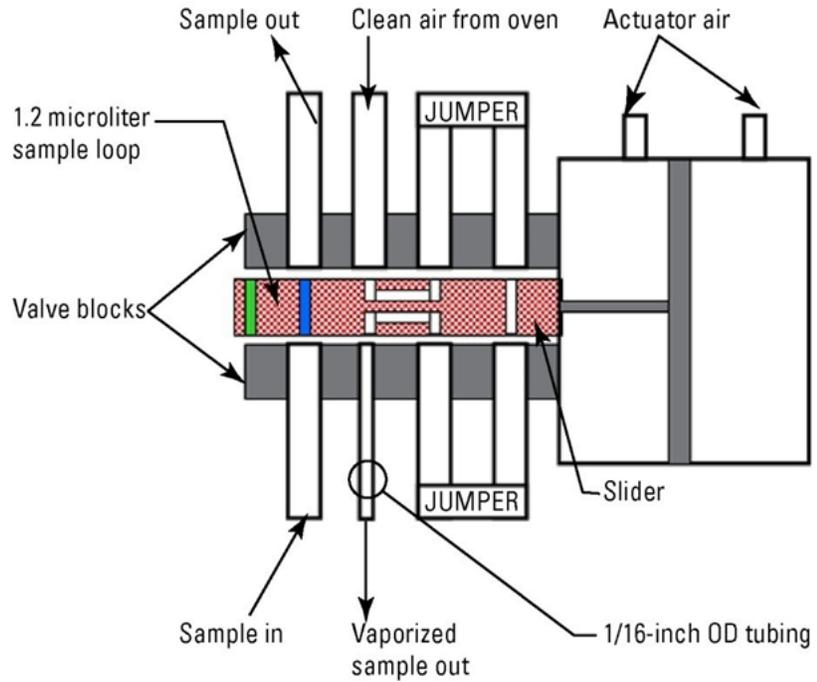
**Figure E-2.** Dinfa 8-port liquid injection valve, sample load position
