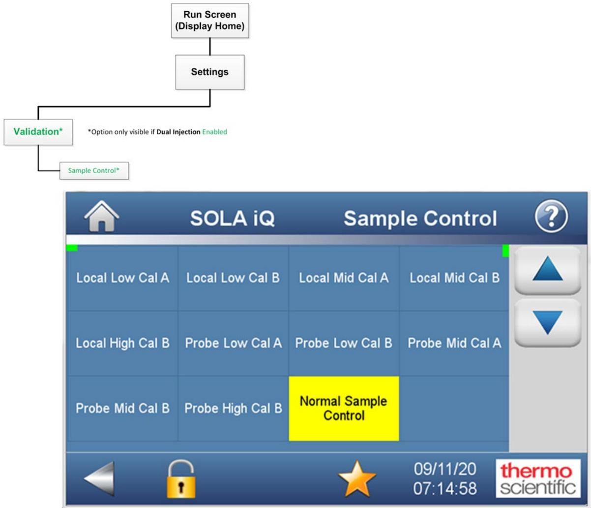
**Figure B-10.** Menu Tree – Validation Sample Control Screen
