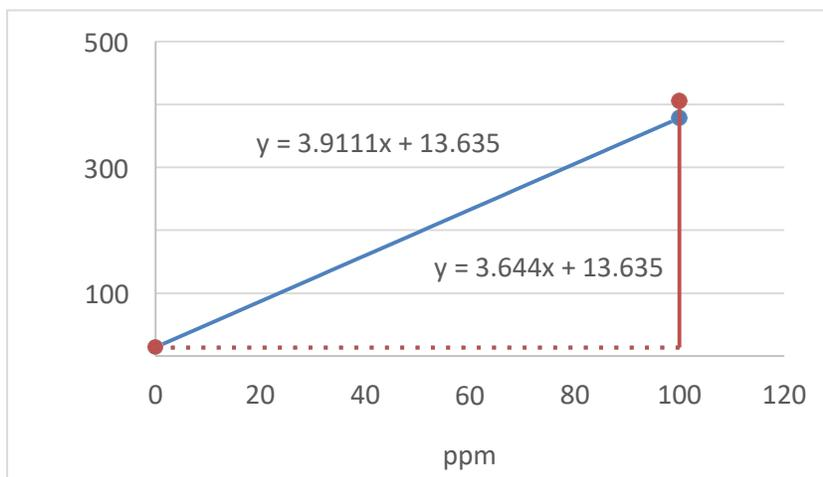
**Figure 5–32.** High calibration
