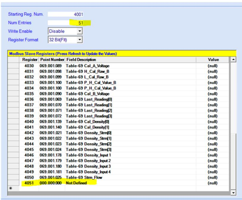
Figure J–3. Modified Modbus Slave Communication Block APP Screen
