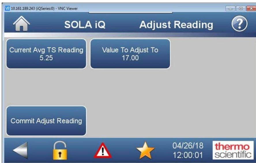
**Figure 5–38.** Adjust Reading screen on Front Panel Display
