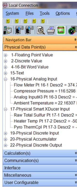
**Figure 4–16.** Navigation Bar – Physical Data Point(s) Selections
