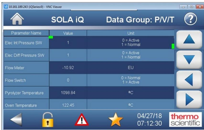
**Figure 4–27.** Pyrolyzer and Oven Temperature Display Values
