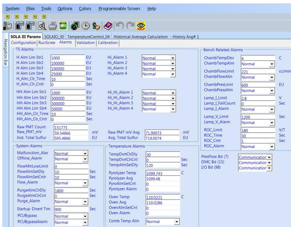
**Figure 4–28.** Bench Related Alarms - Lamp ROC Parameters (far right column)
