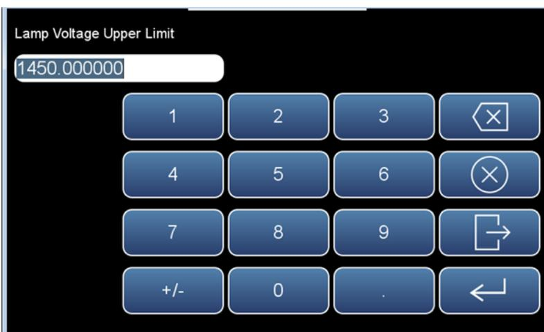
**Figure 5–4.** Display Alarm Set Point Change Screen
