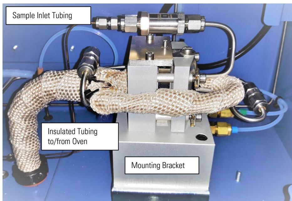
**Figure E-1.** Dinfa Valve mounted in Pneumatics Section
