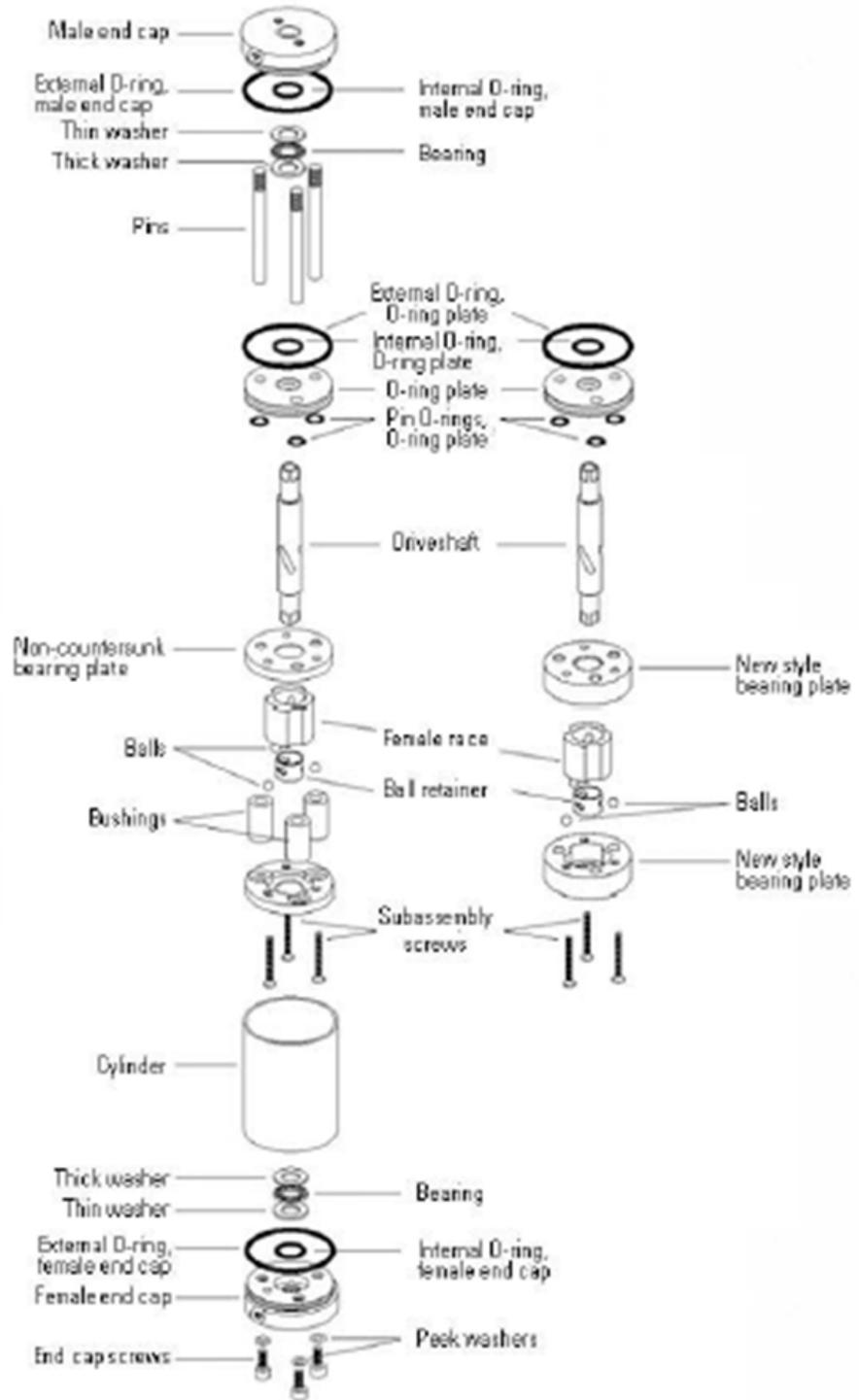
**Figure D-12.** Exploded view of two-position actuator
