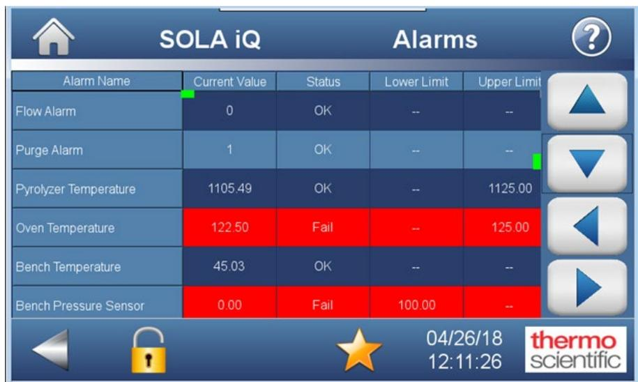
**Figure 6–3.** Alarms page indicating an alarm condition
