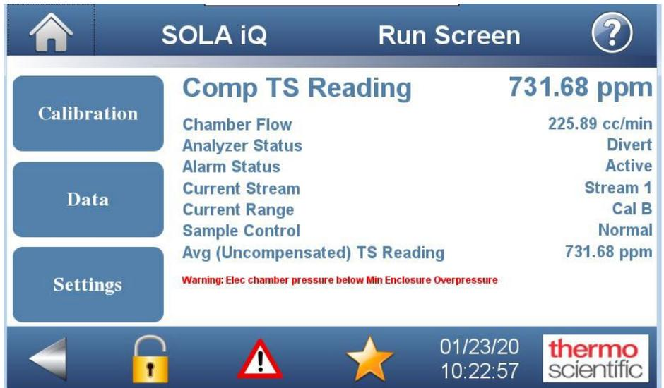
Figure 3-3. Display – Alarm Condition (note red triangle icon)
