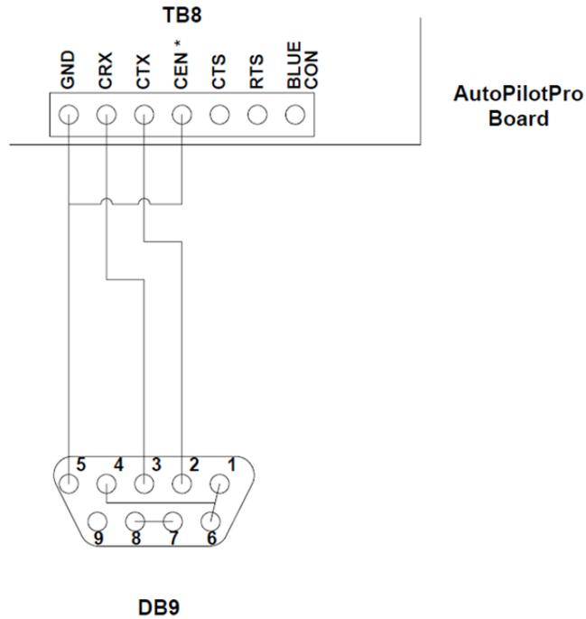
**Note** It is necessary to communicate with the APP board via its serial port NOT through Ethernet. ▲
