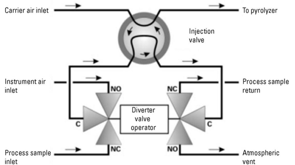
**Figure 4–30.** Sample diverter valves functional diagram (Instrument air inlet is Carrier gas)
