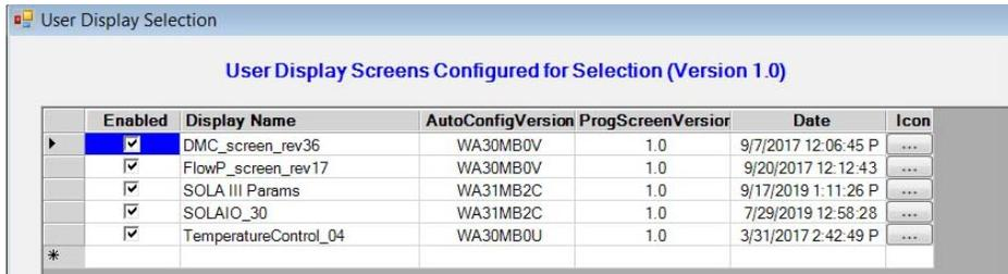
While still in the AutoCFG program, under “Programmable Screen”, check “User Display Screen”. This adds a space populated with user programmable screen icons as shown below, one icon for each XML selected.
