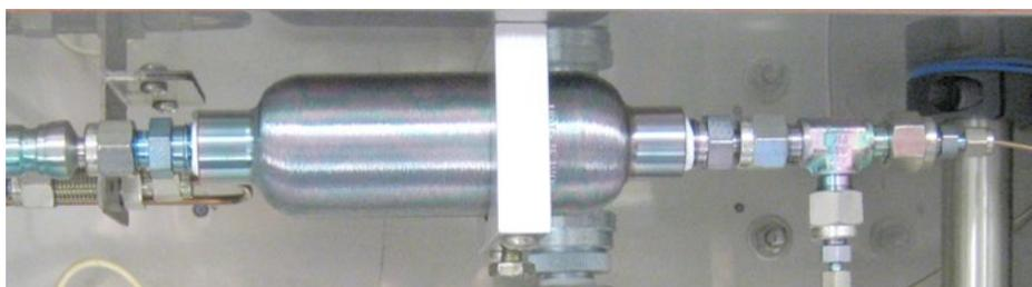
**Figure 2-5.** Typical mixing chamber
