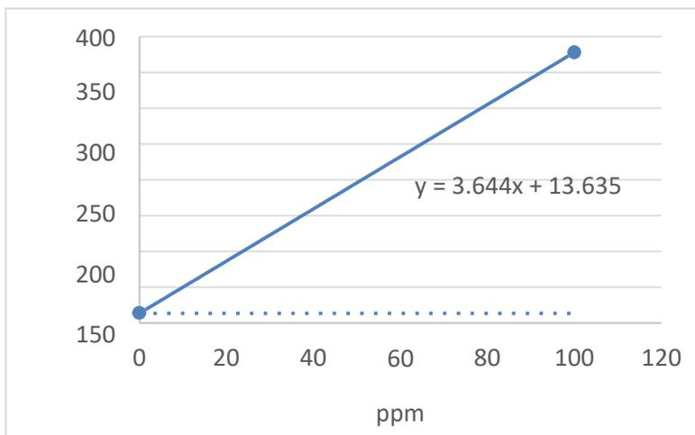
**Figure 5–31.** Typical SOLA iQ calibration
