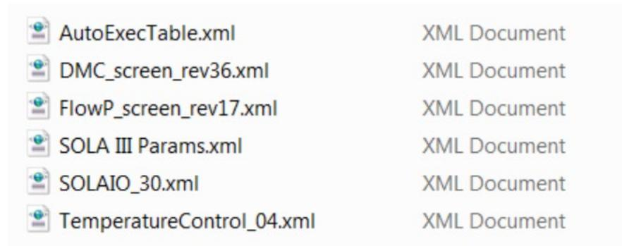
To install these files to the AutoCFG program, copy the "AutoExecTable.xml" to the AutoCFG installation directory, e.g. C:\Thermo\AutoConfig.
