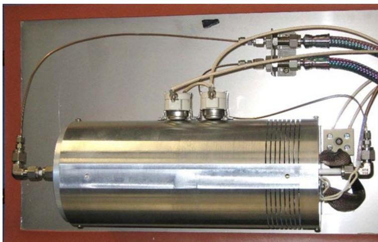
**Figure 8–6.** Pyrolyzer assembly Mounted on Oven Door
