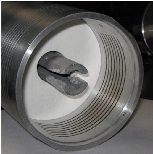
**Figure 8–13.** End view Silicon Carbide Pyrolyzer Heating Element (without electrical connections)
