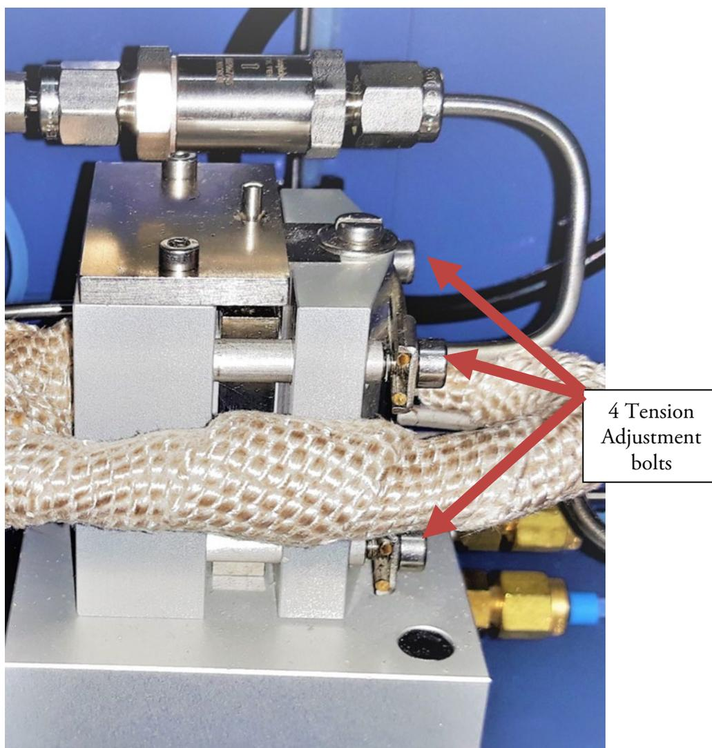
**Figure E-7.** Valve block tension adjustment bolts
