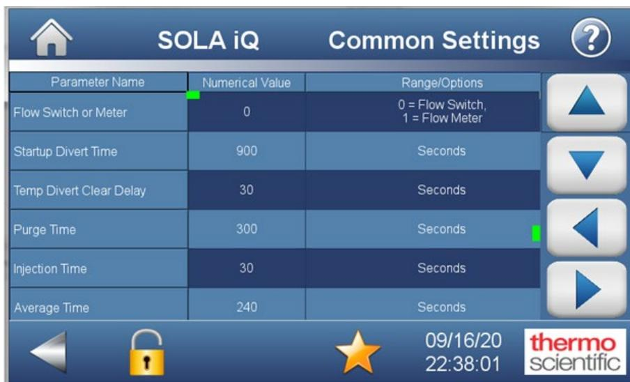
**Figure 5–24.** Common Settings page of the Front Panel Display
