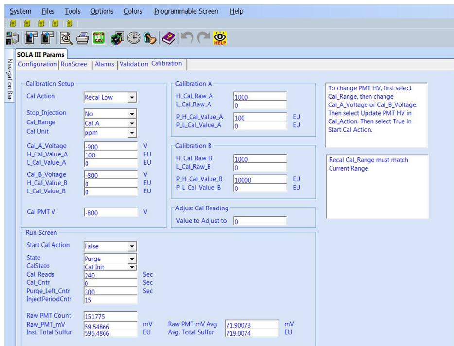
**Figure 5–36.** SOLA iQ Params preconfigured page – Calibration Screen
