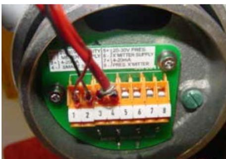
**Figure F–2.** Sarasota FD910 headmount assembly terminal connections
