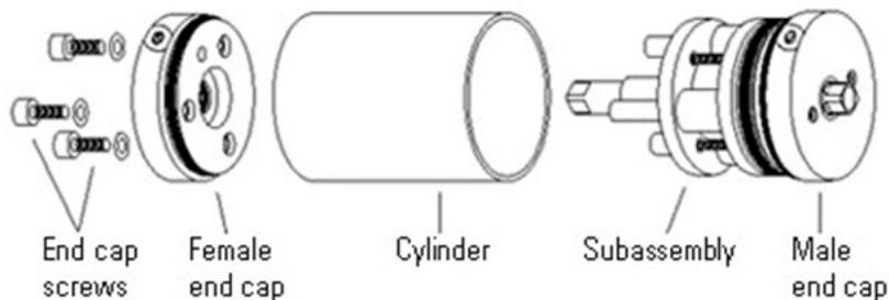
**Figure D-6.** Disassembly Steps 3 through 6
