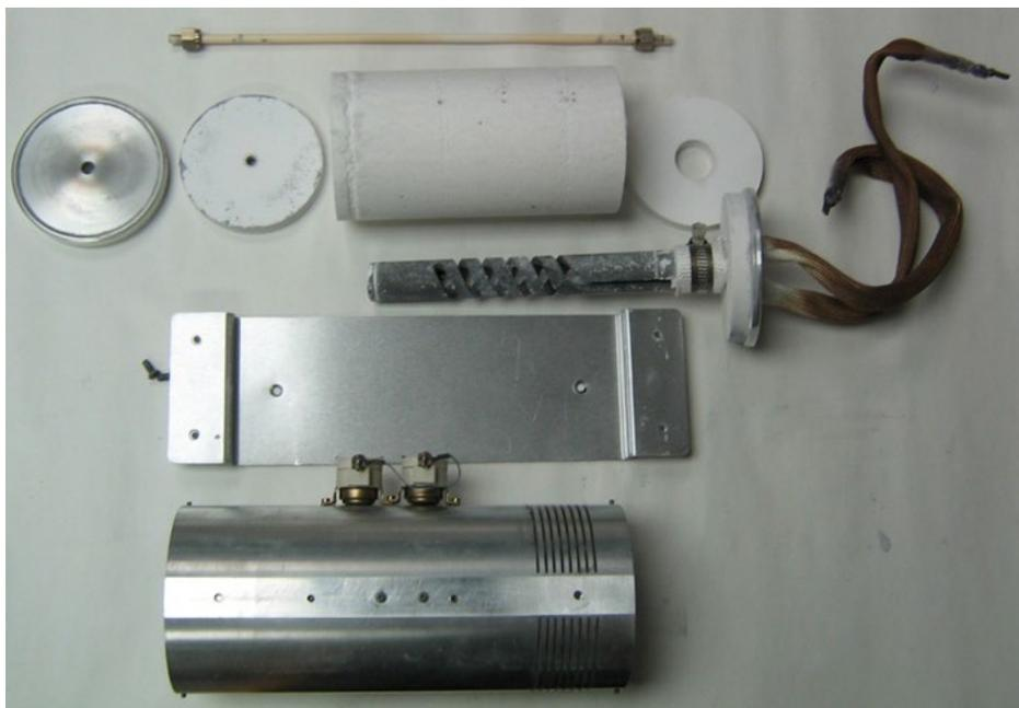
**Figure 8–9.** Disassembled Pyrolyzer
