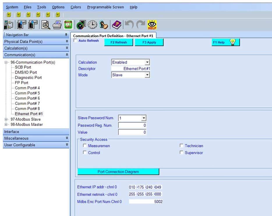
To change the Ethernet Static IP address, enter a new valid address at Ethernet IP addr - chnl 0. Change the Ethernet gateway - chnl 0 to match the desired network address. Press F3 Apply and perform a Warm Start (select Tools - Warm Restart) to enable the changes.
