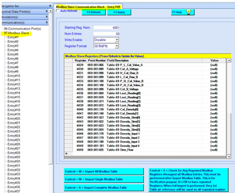
Figure J–2. Modbus Slave Communication Block APP Screen
