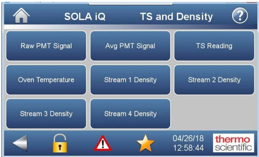
Figure 7-5. View Parameters II > TS and Density
