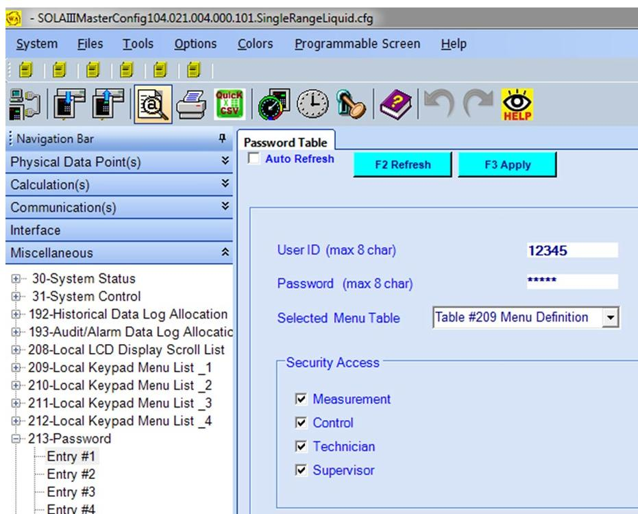
To set a password in the AutoPilot Pro, enter your desired User ID and Password and select which access levels will be password protected. In the example shown above, all access levels will be password protected.
