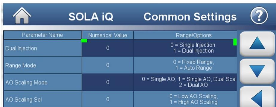
The SOLA iQ may have up to two calibration ranges available. These are designated as CAL A and CAL B. The Range Mode option allows each stream to be assigned a calibration range in Fixed Range Mode or lets the SOLA iQ automatically select the range in Auto Range Mode.
