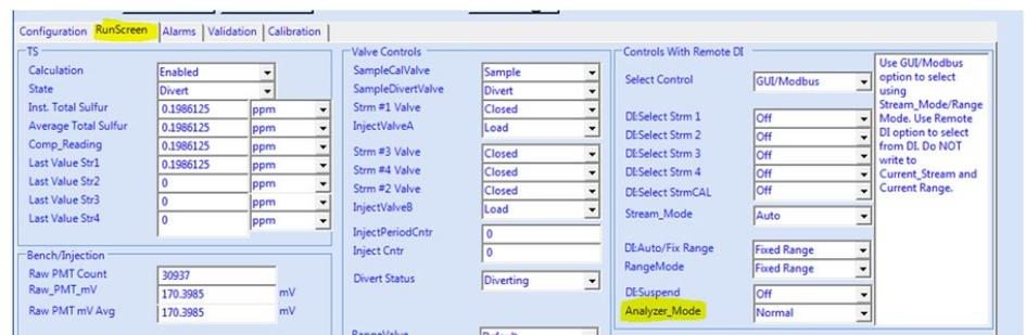
**Figure J-6.** Analyzer\_Mode box on Run Screen in SOLA III Params
