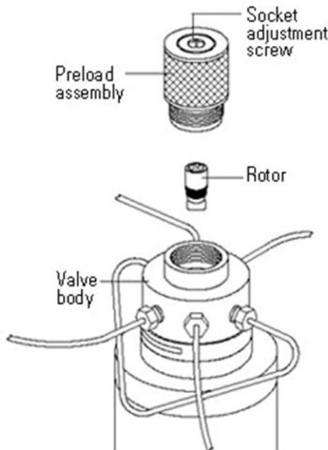
**Figure D-1.** Rotary valve disassembly
