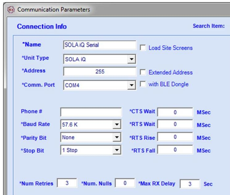
4. Start AutoConfig on the PC/Laptop & connect to the APP board.
