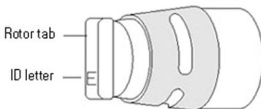
**Figure D-3.** Location of ID letter on valve rotor
