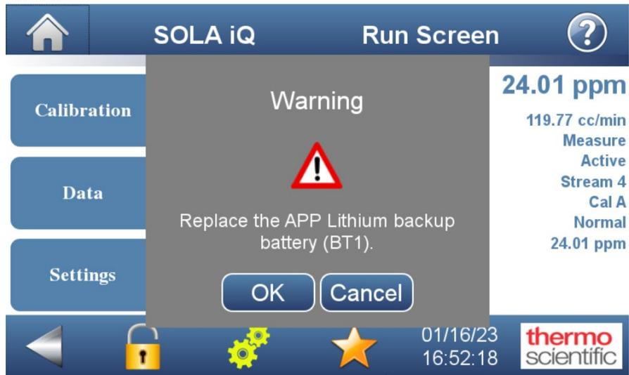
**Figure H-2.** Replace Lithium backup battery warning
