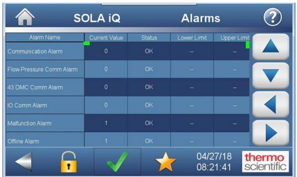
Figure 3-4. Display – No Alarm Condition (note green checkmark)
