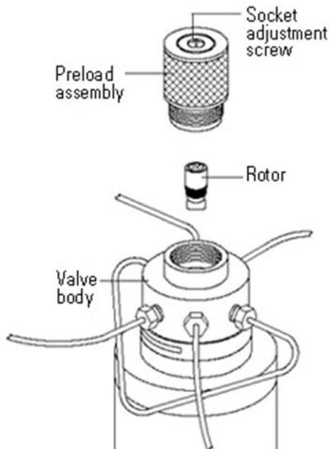
**Figure D-1.** Rotary valve disassembly
