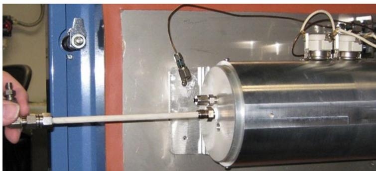
**Figure 8–11.** Remove Pyrolyzer Reaction Tube
