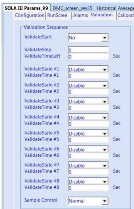
Figure 5–11. Validation Setup Screen
