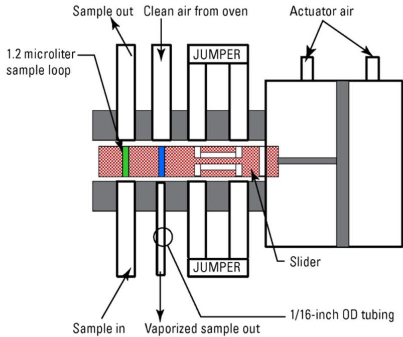
**Figure E-3.** Dinfa 8-port liquid injection valve, inject position
