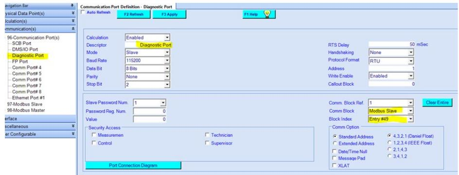
**Figure J-1.** Diagnostic Port of the Communication Port Definition APP Screen
