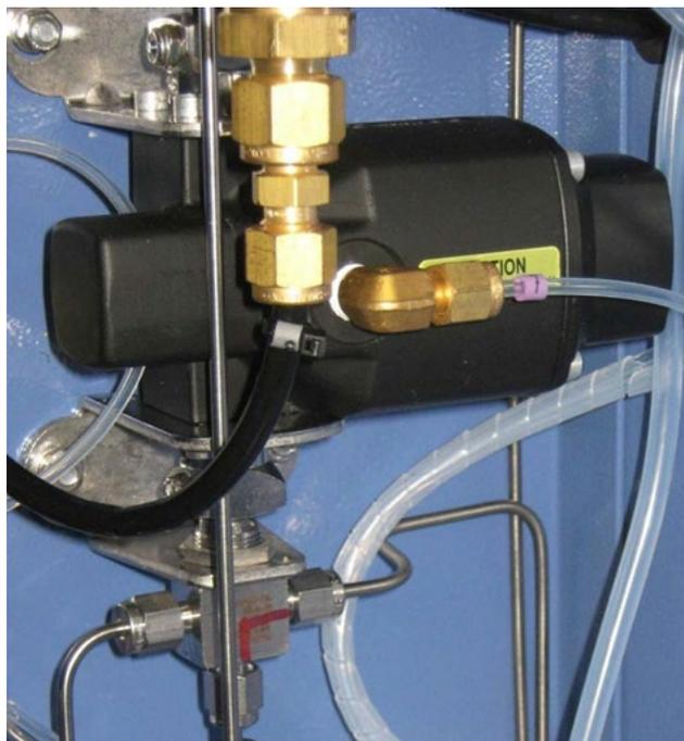
**Figure 4–29.** Sample diverter valves
