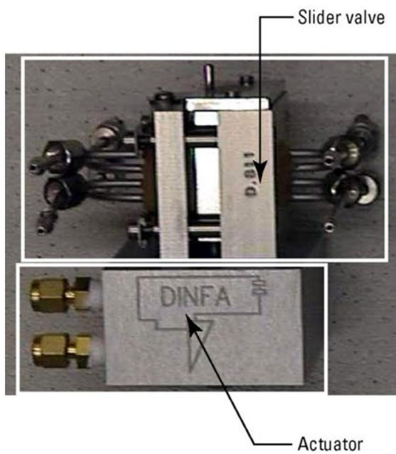
**Figure E-5.** Dinfa 8-port liquid injection valve
