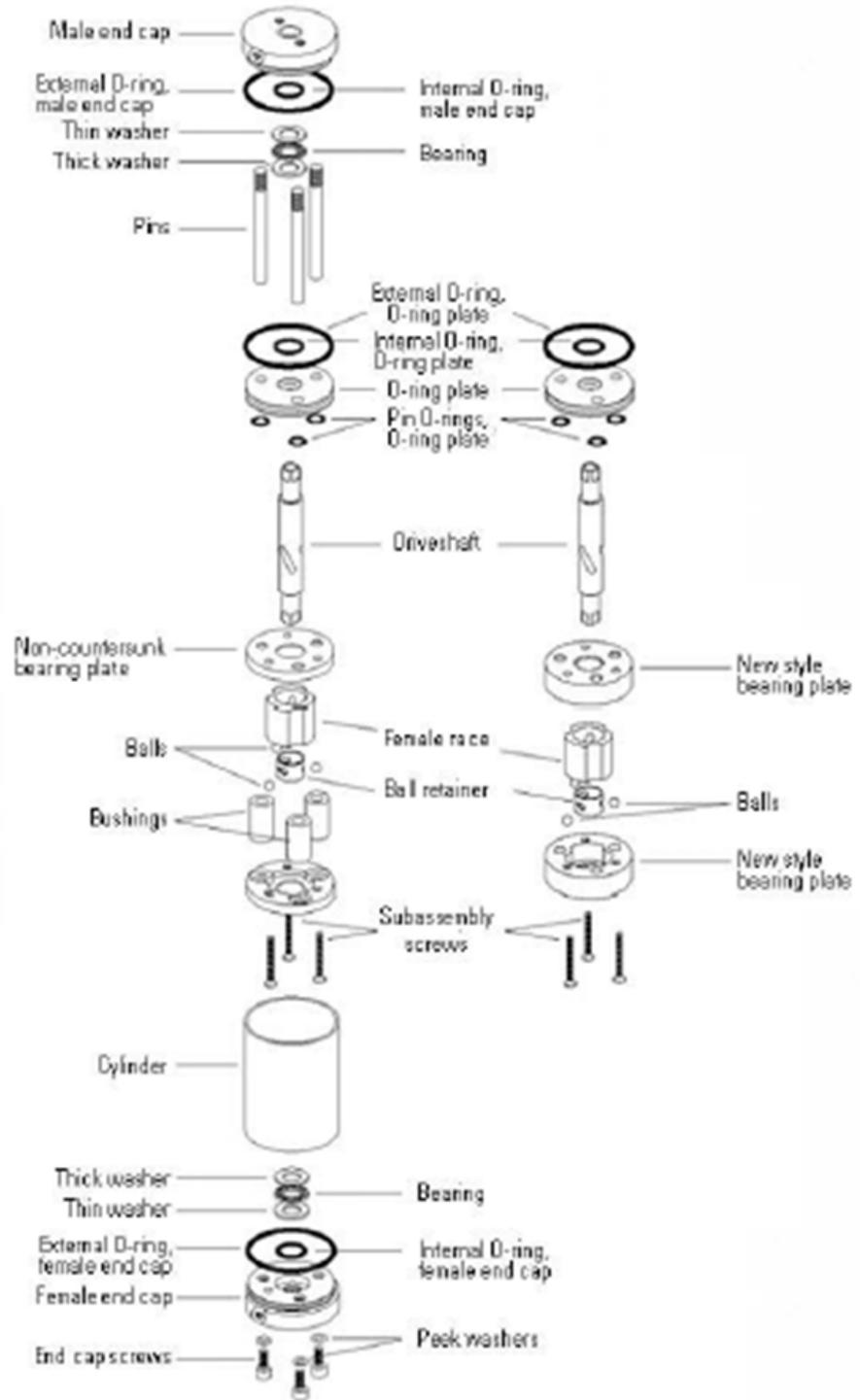
**Figure D-12.** Exploded view of two-position actuator
