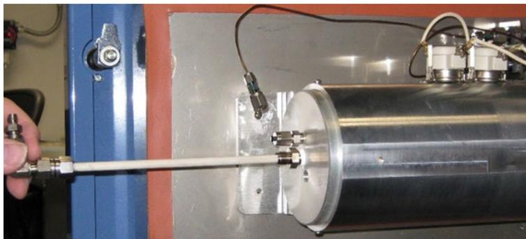
**Figure 8–17.** Pyrolyzer tube removed/inserted through fitting
