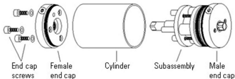
**Figure D-6.** Disassembly Steps 3 through 6
