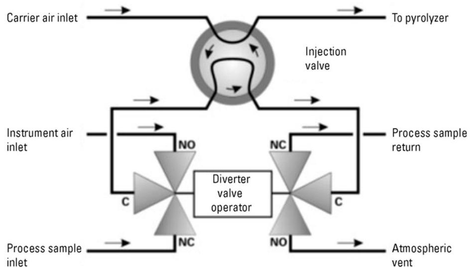
**Figure 4–30.** Sample diverter valves functional diagram (Instrument air inlet is Carrier gas)
