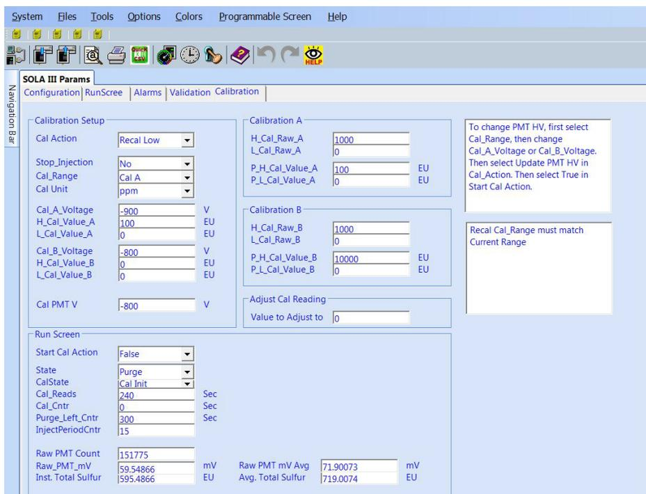
**Figure 5–26.** Calibration page of SOLA\_III\_Param preconfigured screen in Auto CONFIG
