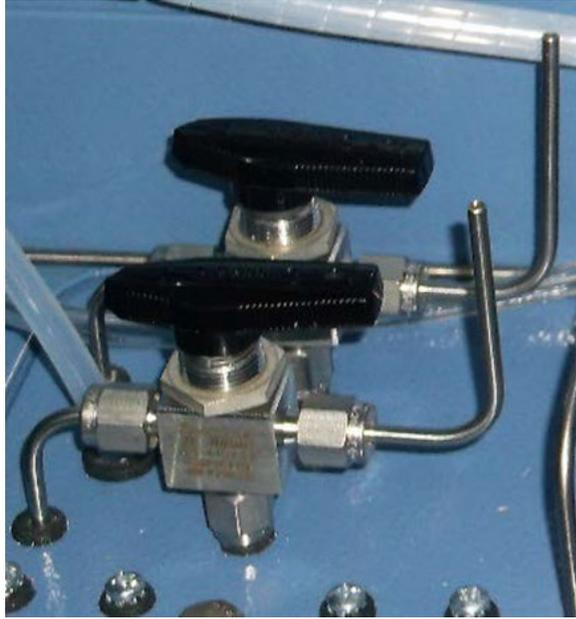
**Figure 8–4.** Three-way measure Valve
