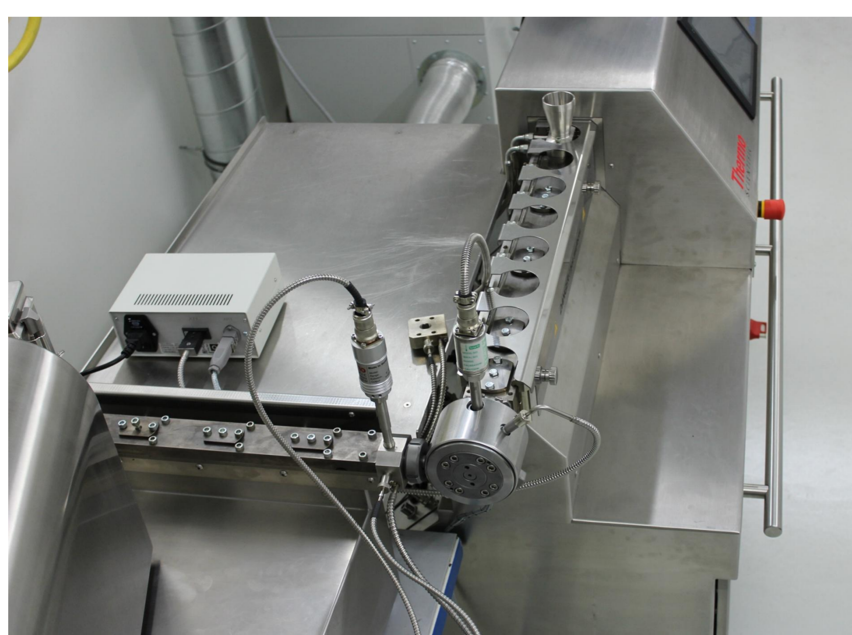
FIGURE 1: set up of twin screw extruders for co-extrusion
