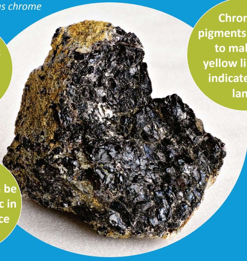
Chromite, (pictured) an oxide of iron, magnesium, aluminum, and chromium, is the only ore mineral of chromium.
