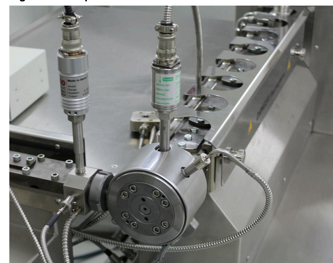
Figure 1. Set-up of Extruders for Co-Extrusion
