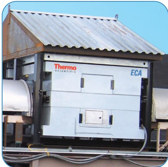
The Thermo Scientific Elemental CrossBelt Analyzer (ECA) is used to control the sorting and blending of coals to maximize coal resources, reduce out-of-seam dilution and control preparation plant performance. The analyzer is designed for applications requiring process accuracy at a modest cost.
