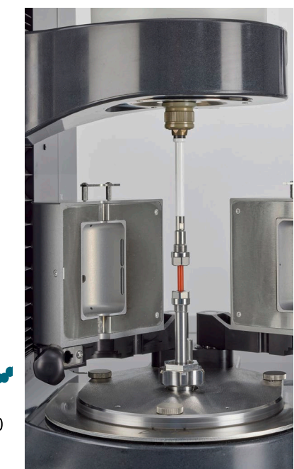
DMTA thermogram of two different filaments with different API content (left) as well as the used rheometer configuration (right)
