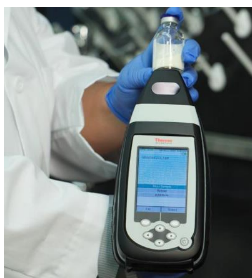
Thermo Scientific microPHAZIR RX Analyzer can provide raw material identification in seconds.
