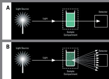
Figure 2 Differences between forward and reverse optical systems.
