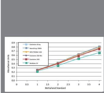
**Figure 6** Comparison of OD data measured on standard spectrophotometers and a spectrophotometer with an ISA. The OD600 of various McFarland standards was measured on an Evolution 260 Bio (dark blue), NanoDrop 2000c (light blue), and with an integrating sphere accessory (black). Significant differences in absorbance values were observed between the spectrophotometer with the ISA and standard instruments.
