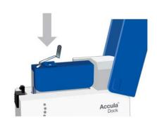
Once the sample is ready to be inserted, Remove foil tab covering sample port on Test Cassette and discard
