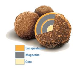
This SEM image shows the unique cauliflowerlike surface of the Sera-Mag Speedbeads which dramatically increases the overall surface area available for binding. Sera-Mag SpeedBeads also have a second layer of magnetite within the particle, resulting in a 2x faster increase in speed in response to magnetic field.
