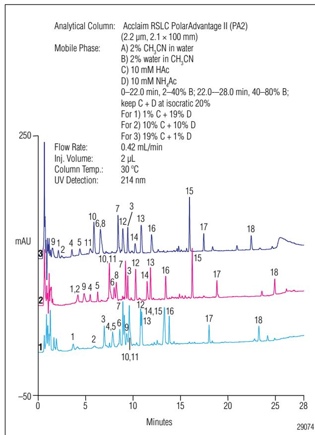
Figure 3. Peptide mapping of myoglobin on the Acclaim RSLC PA2 column at pH 5.6 (1), pH 3.7 (2) and pH 2.9 (3).
