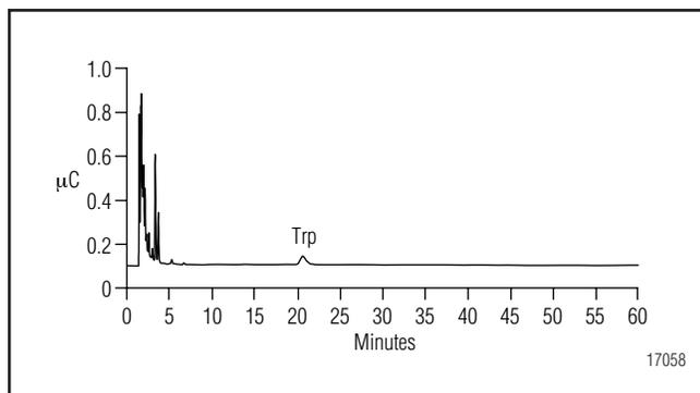
Figure 10. Determination of 6.5  $\mu\text{M}$  Trp in YPD broth (100-fold dilution, 500  $\mu\text{g}/\text{mL}$ , 25  $\mu\text{L}$  injection) using Method 1.
