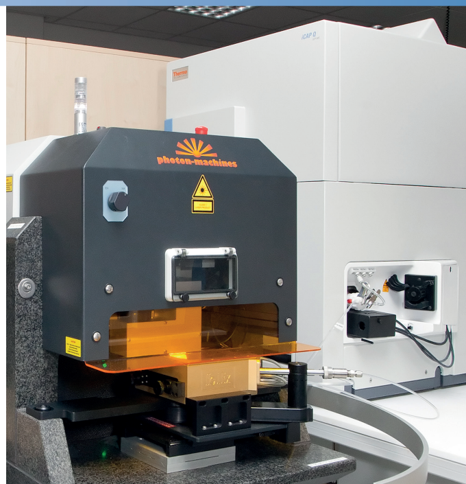
Figure 1: The Photon Machines Analyte G2 laser ablation connected to the Thermo Scientific iCAP Q ICP-MS
