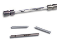
Figure 2. Thermal desorption glass tubes used for VDA 278 analysis with a prepared sample.
