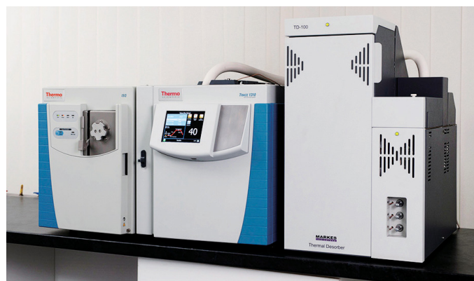
Figure 1. Automated thermal desorption system with GC-MS detection for VDA 278 analysis, comprised of a Thermo Scientific TRACE 1310 GC system, a Thermo Scientific ISQ LT single quadrupole GC-MS system and a Markes TD100 Thermal Desorber.
