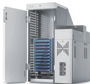
Figure 3. Detail of the automated thermal desorption system loaded with sample tube trays (Markes TD-100).
