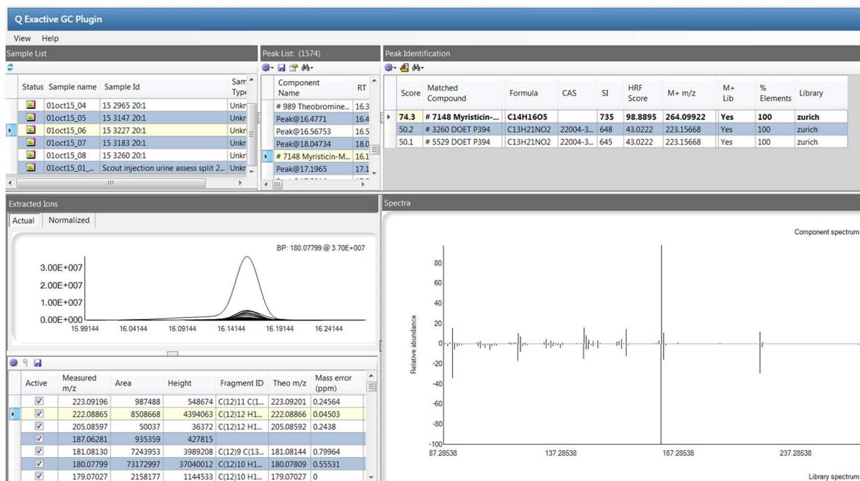
Figure 3. Identification of myristicin using TraceFinder. Spectral deconvolution of the TIC and library search index and the HRF score together with additional criteria are used for intelligent compound identification. The list of matched compounds (upper) is sorted based on a combined search index and high resolution filtering (HRF) score.
