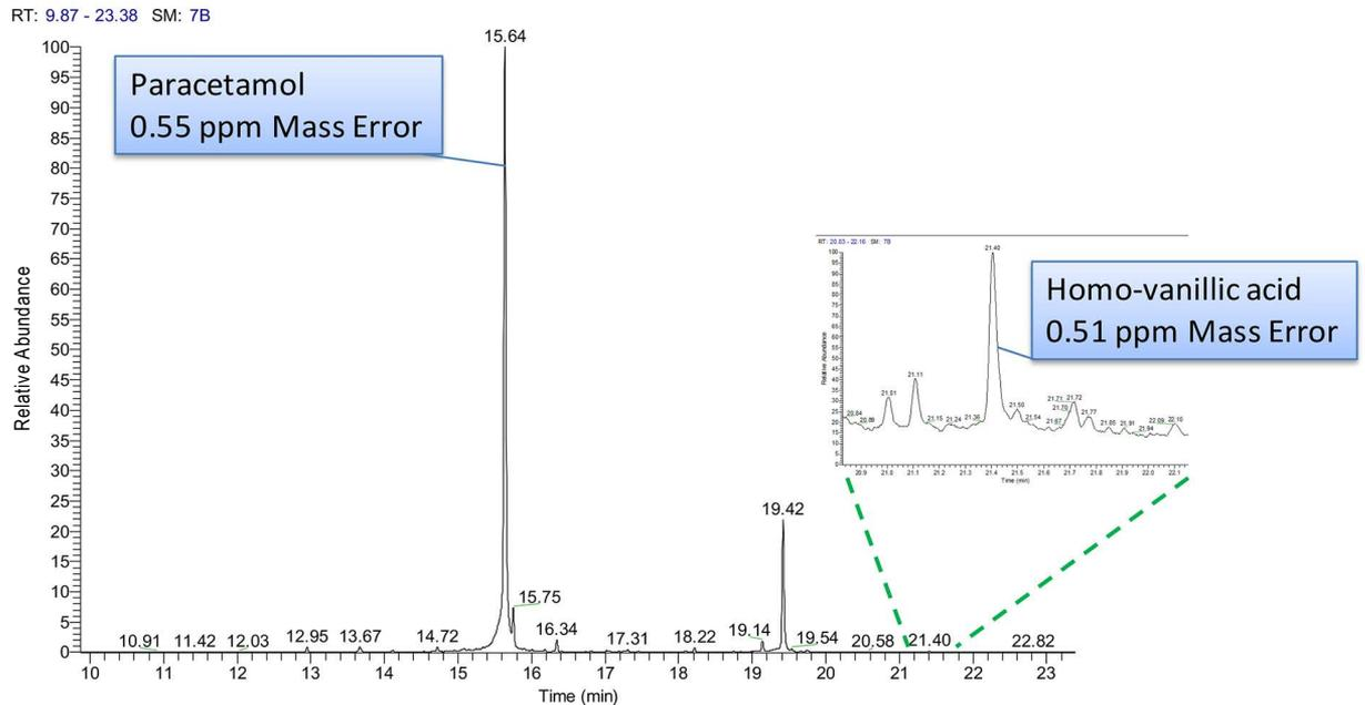
Figure 5. Mass accuracy at sub 1 ppm regardless of compound concentration. Paracetamol (0.5 ppm for BP  $m/z$  109.05221) peak area 930 times higher than homo-vanillic acid (0.5 ppm for BP  $m/z$  137.0597).
