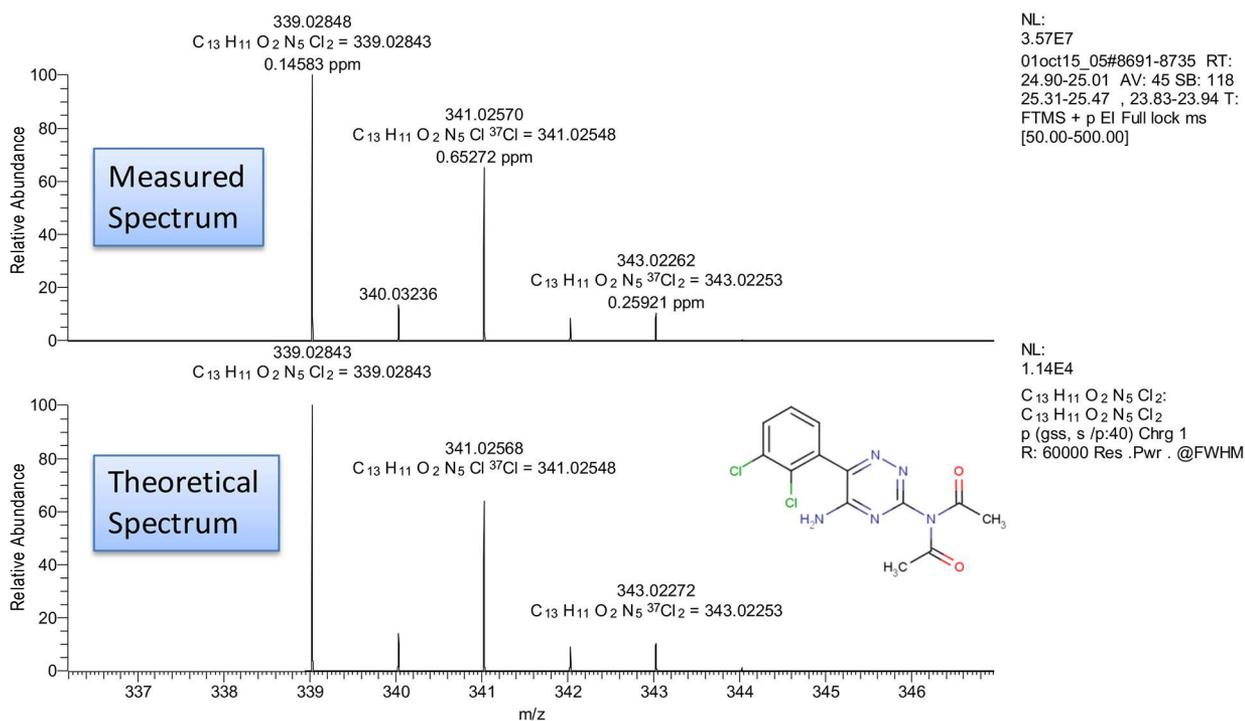
Figure 4. Measured and theoretical isotope molecular ion cluster of lamotrigine 2AC. Elemental formula for each isotope is displayed with in each case < 1 ppm mass accuracy.
