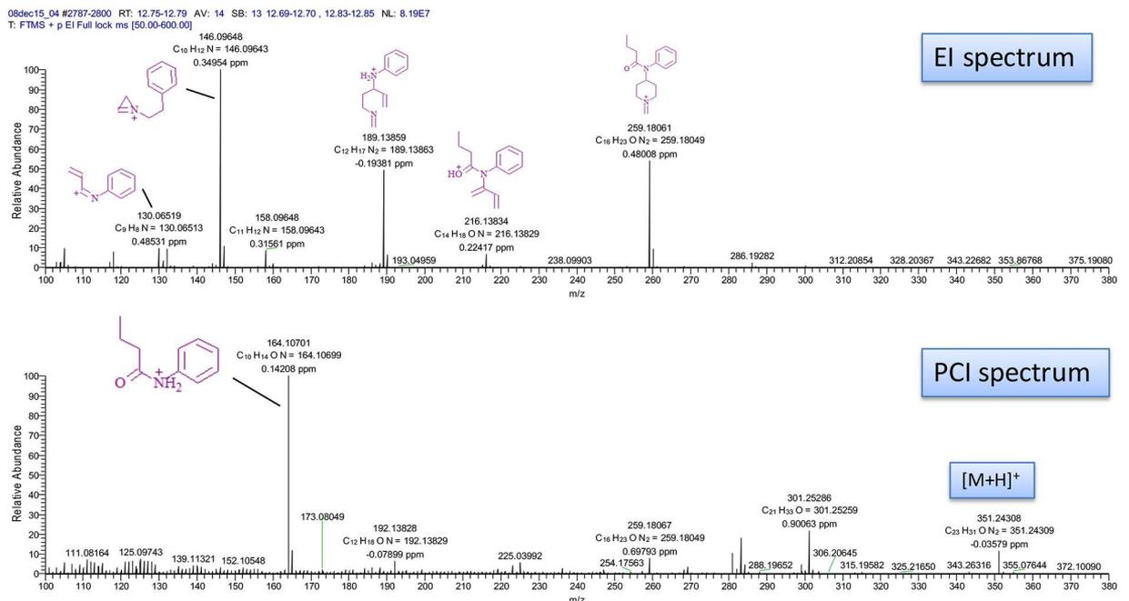
Figure 6. Butyrfentanyl ( $C_{23}H_{30}N_2O$ ) EI and PCI spectra at 12.77 minutes sample F. PCI data supports identification of parent with formula above with sub 1 ppm mass accuracy. EI Fragments annotated with structures from MassFrontier 7.0.
