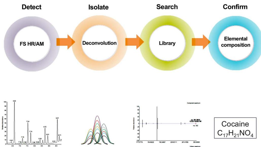
Figure 1. Workflow for the Q Exactive GC system for screening
