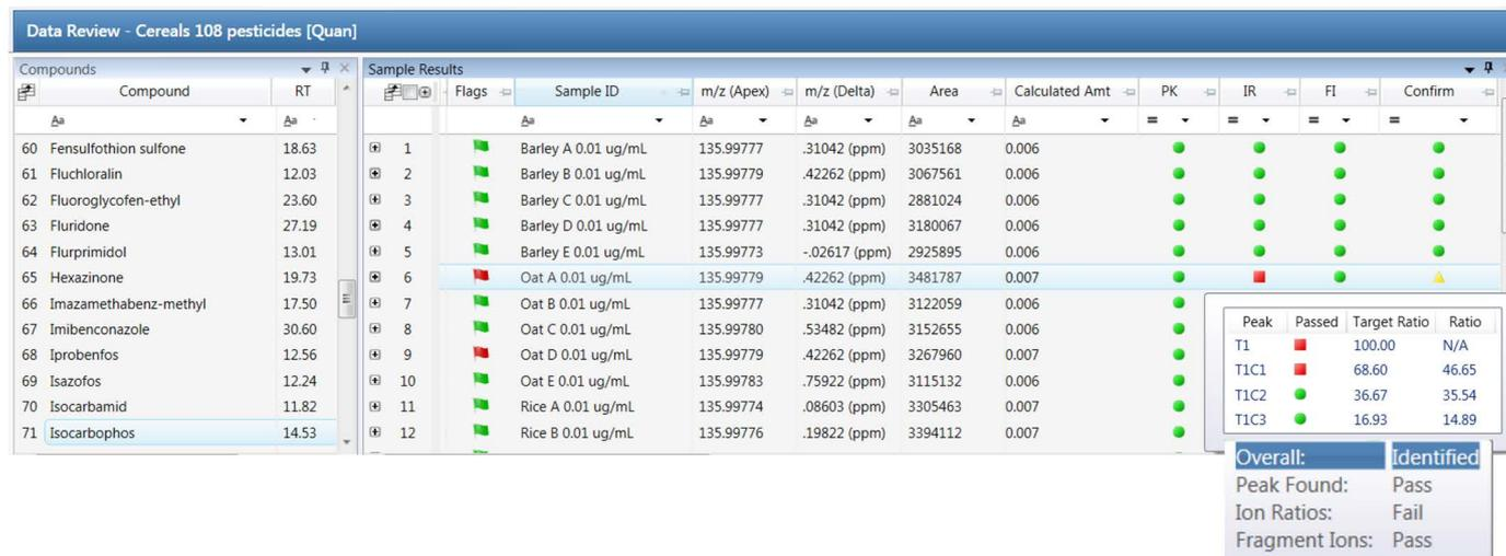
**Figure 2. TraceFinder software browser enables fast data review and confirmation.** The software quickly points the analyst to the data that supports a positive identification using a traffic light system along with real data values. More importantly, it will flag when a parameter is outside of tolerance, and by what value, and allow the analyst to make the final decision to confirm an identification. Hovering above the red square (below) brings up further details.
