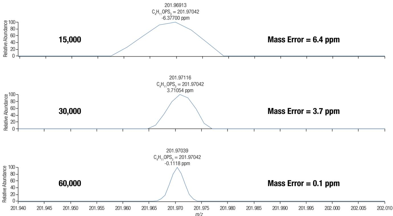
**Figure 6. Effect of resolving power on mass accuracy of diagnostic ion ( $m/z$  201.97042) tribufos at 20  $\mu\text{g}/\text{kg}$  in oat acquired at different resolutions of 15K, 30K, and 60K.**
