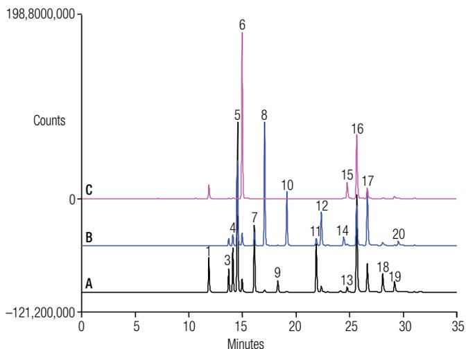
Figure 2. All 20 PAHs (50 µg/L for each PAH) detected by fluorescence detection using programmed wavelength switching in three parallel channels: (A) Emission\_1, (B) Emission\_2, (C) Emission\_3. Note: Acenaphthylene (Peak 2) is not shown here because there was no fluorescent response for acenaphthylene.
