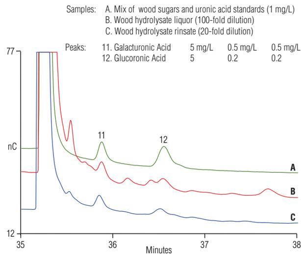
Figure 3. Separation (35–38 min) of two uronic acids using Method 1 on the Dionex CarboPac PA200 column in (A) a mix of standards and (B and C) wood hydrolysate samples. Conditions are the same as in Figure 2.
