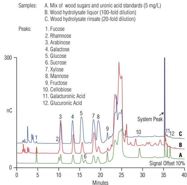
Figure 2. Separation of 10 wood sugars and two uronic acids using Method 1 on the Dionex CarboPac PA20 column in (A) a mix of standards and (B and C) wood hydrolysate samples.
