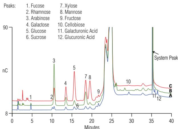
Figure 1. Separation of 10 wood sugars and two uronic acids using Method 1 on the Dionex CarboPac PA20 column in (A) a mix of standards and (B and C) wood hydrolysate samples.
