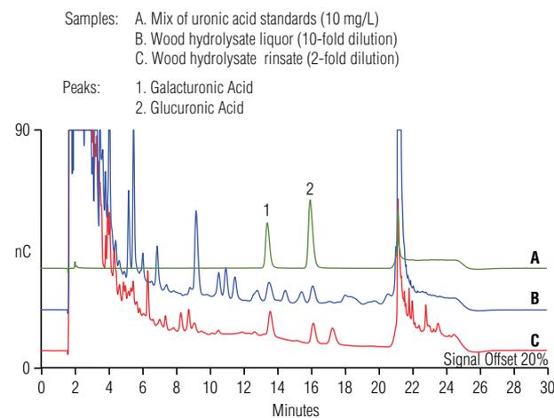
Figure 4. Separation of uronic acids using Method 2 on the Dionex CarboPac PA200 column in (A) a mix of standards and (B and C) wood hydrolysates.
