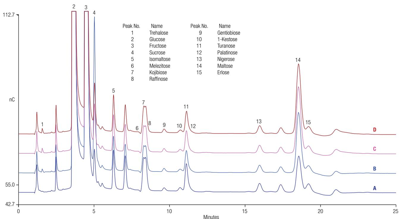
Figure 9. Chromatogram of (A), 100% honey sample (HS1); (B), 80% HS1 adulterated with sugar syrup 1 (+ 20% SS1); (C), 80% HS1+ 20% SS2; and (D), 80% HS1+ 20% SS3.
