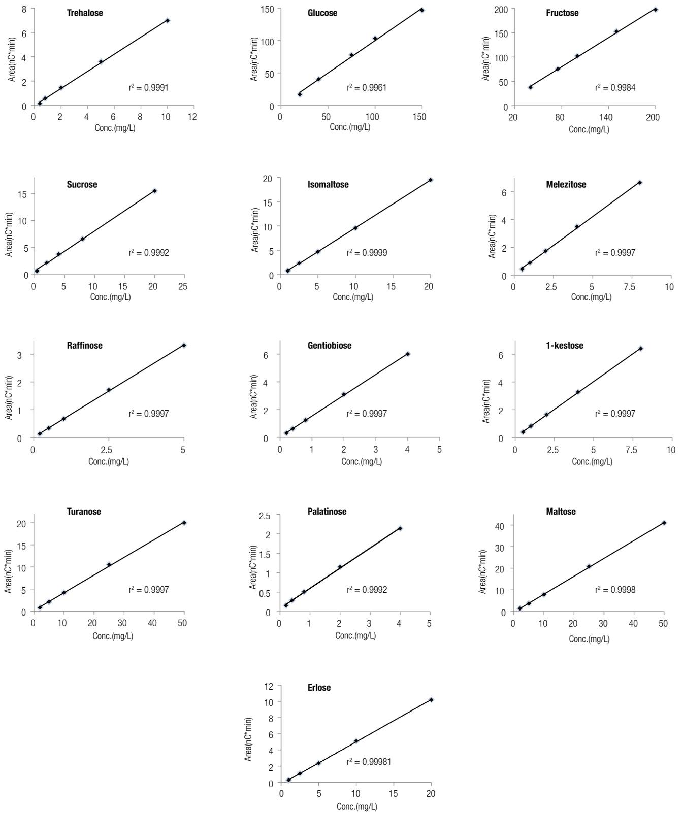
Figure 7. Calibration curves of 13 honey sugar standards.
