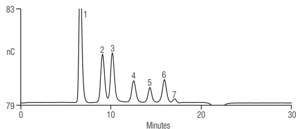
Figure 2. Separation of *meso*-erythritol, glycerol, propylene glycol, ethanol, methanol, and isopropanol.
