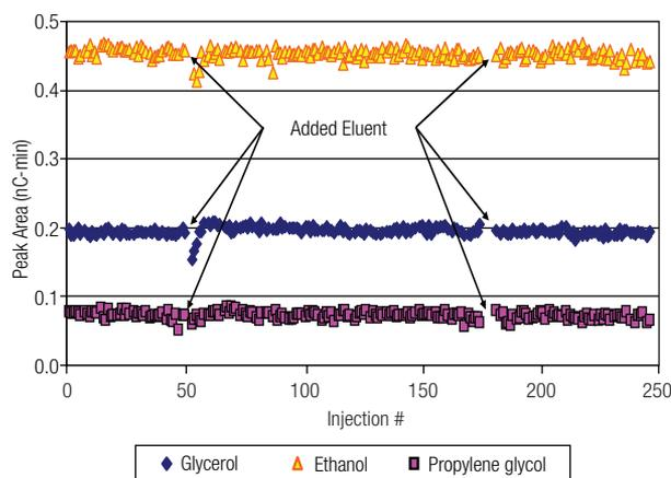
Figure 5. Peak area stability of 50  $\mu\text{M}$  glycerol, propylene glycol, and ethanol spiked into a 300-fold dilution of the supernatant from heat quenched and centrifuged American Wheat *S. cerevisiae* incubated in Bacto YPD.
