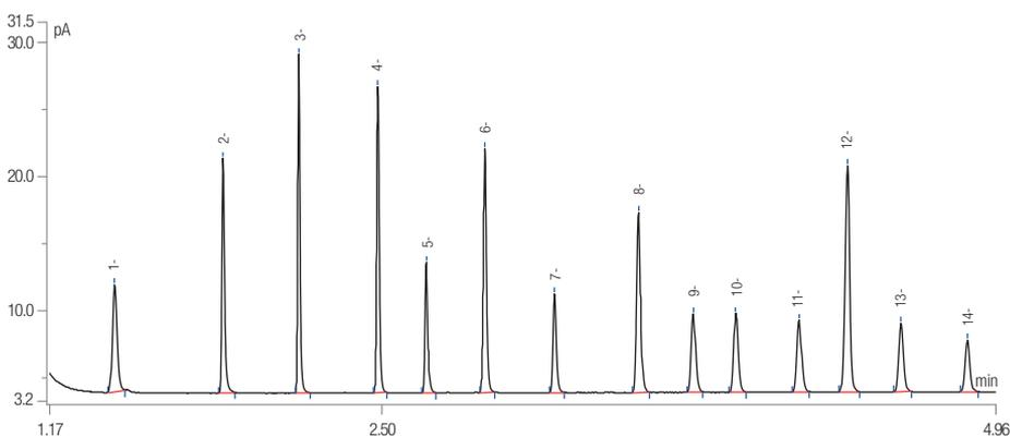
**Figure 4b (peaks 1–14).** Fast analysis on a TRACE TR-FAME GC column 10 m × 0.10 mm × 0.2 μm with hydrogen carrier gas. (Experiment 2)
