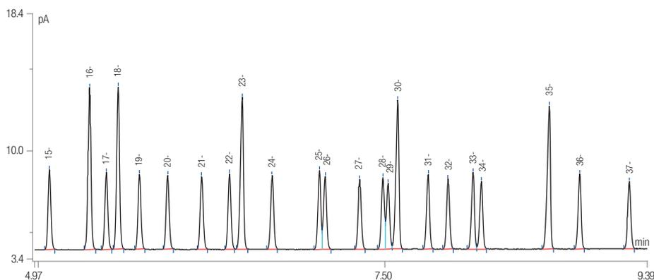
**Figure 4c (peaks 15–37).** Fast analysis on a TRACE TR-FAME GC column 10 m × 0.10 mm × 0.2 μm with hydrogen carrier gas. (Experiment 2)
