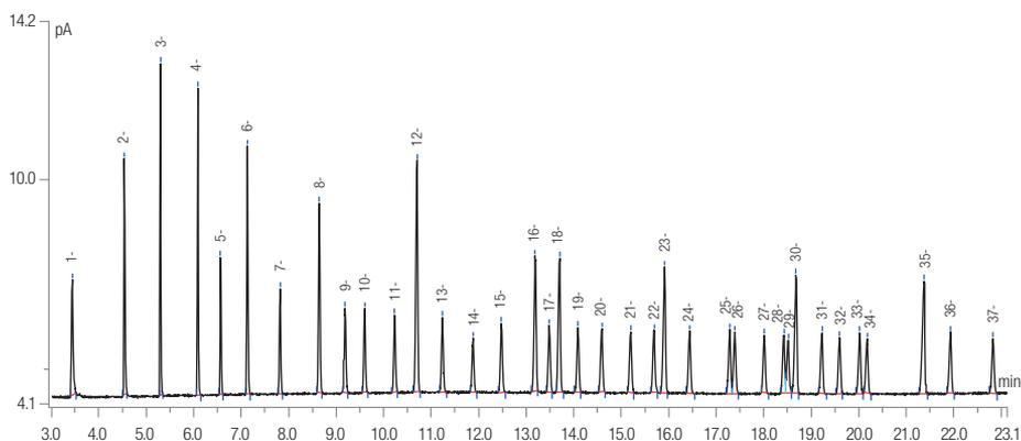
Figure 6a (full chromatogram nitrogen). Analysis on a TRACE TR-FAME GC column 10 m × 0.10 mm × 0.2 μm cyanopropyl phase using nitrogen carrier gas. (Experiment 3)
