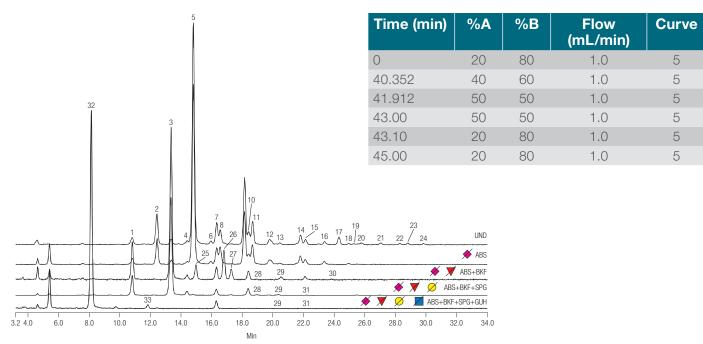
Figure 3. HILIC chromatograms of the infliximab 2-AA labeled N-glycan pool (undigested, UND) and after digestion with a range of exoglycosidase enzymes. Separations were performed on an Accucore 150-Amide-HILIC 2.1 × 150 mm column using the gradient conditions outlined in the figure legend table.
