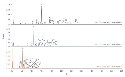
Figure 2. Chromatographic separation of commercial chimeric IgG1 mAb (infliximab) 2-AA-labeled *N*-glycans on Accucore 150-Amide-HILIC columns of varying lengths.
