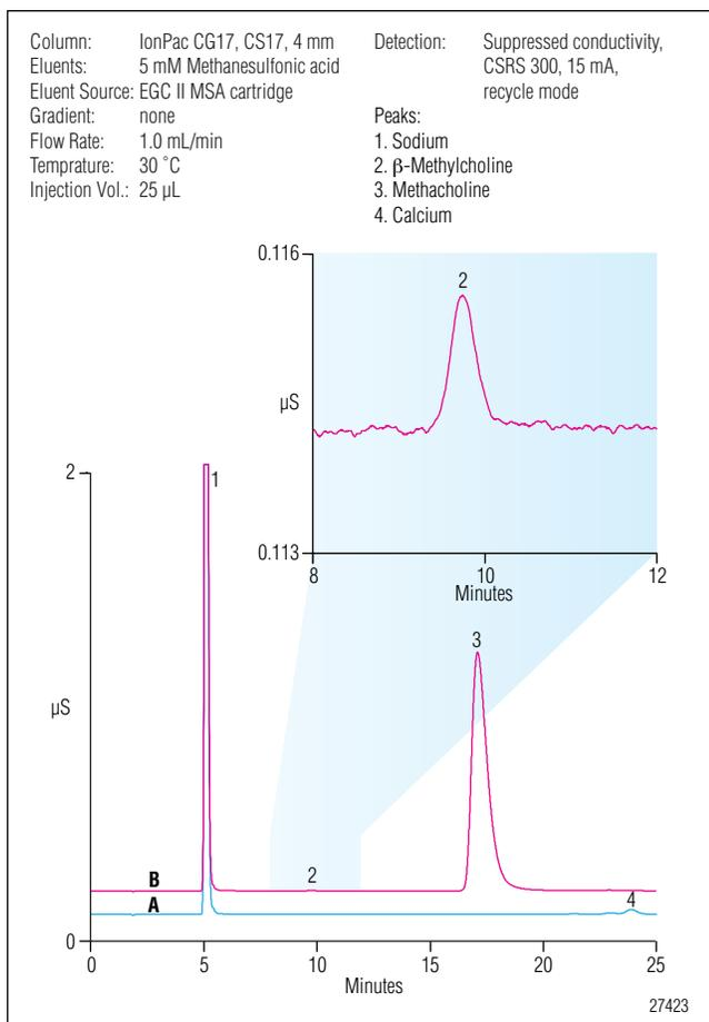
Figure 3. Cations in 1000:1 dilution in 0.9% NaCl + 0.4% phenol matrix. Trace A, matrix blank; trace B, 25 mg/L methacholine in diluted matrix ( $\beta$ -methylcholine conc.  $\sim$  0.1% of methacholine). The inset shows the 8 to 12 min region.
