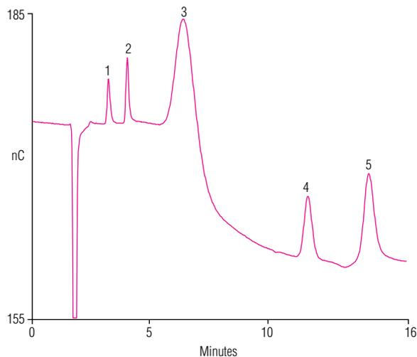
Figure 2. Mixed aminocarboxylate chelate standard separated and detected by anion-exchange chromatography with pulsed amperometric detection.
