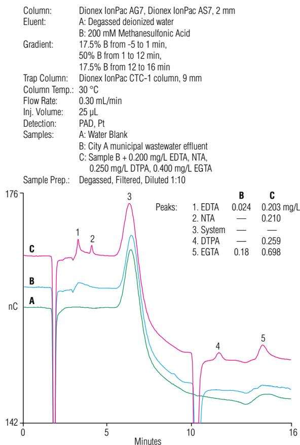
Figure 4. Comparison of 1:10 dilution of City A municipal wastewater effluent B) without and C) with chelates added.
