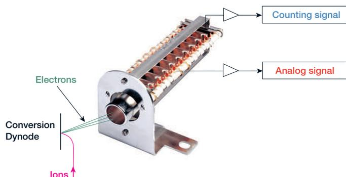
Figure 1. Element 2 HR-ICP-MS Ion Detection System.
