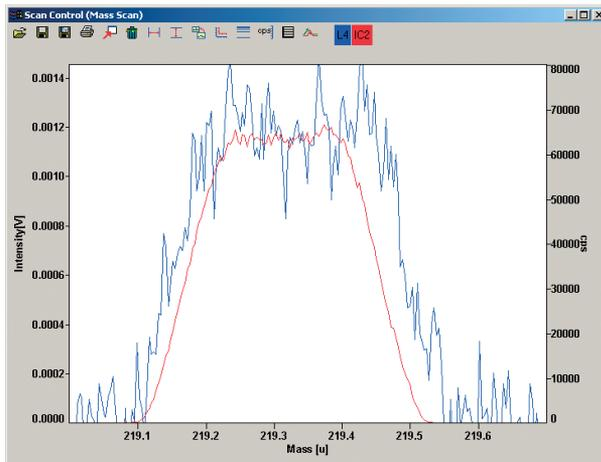
Figure 1. Multicollector measurement of the isotopes  $^{206}\text{Pb}$  and  $^{207}\text{Pb}$  from a SRM 981 standard at 200 ppt concentration. Signal intensities of both isotopes are similar and yield about 1.2 mV on Faraday cup L4 (blue), respectively 65,000 cps on ion counter IC2 (red).
