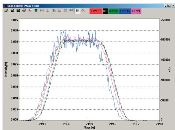
Figure 2. Typical peak shape and peak overlap of the U and Pb isotope signals detected on the ion counters.
