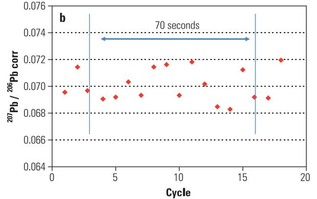
Figure 6a. Intensity profile of  $^{206}\text{Pb}$  during ablation of 91500. Figure 6b. Stability of  $^{207}\text{Pb}/^{206}\text{Pb}$  (corrected for common Pb) during the ablation process. The average  $^{207}\text{Pb}/^{206}\text{Pb}$ corr = 0.069942 (1 s.e. = 0.45%).
