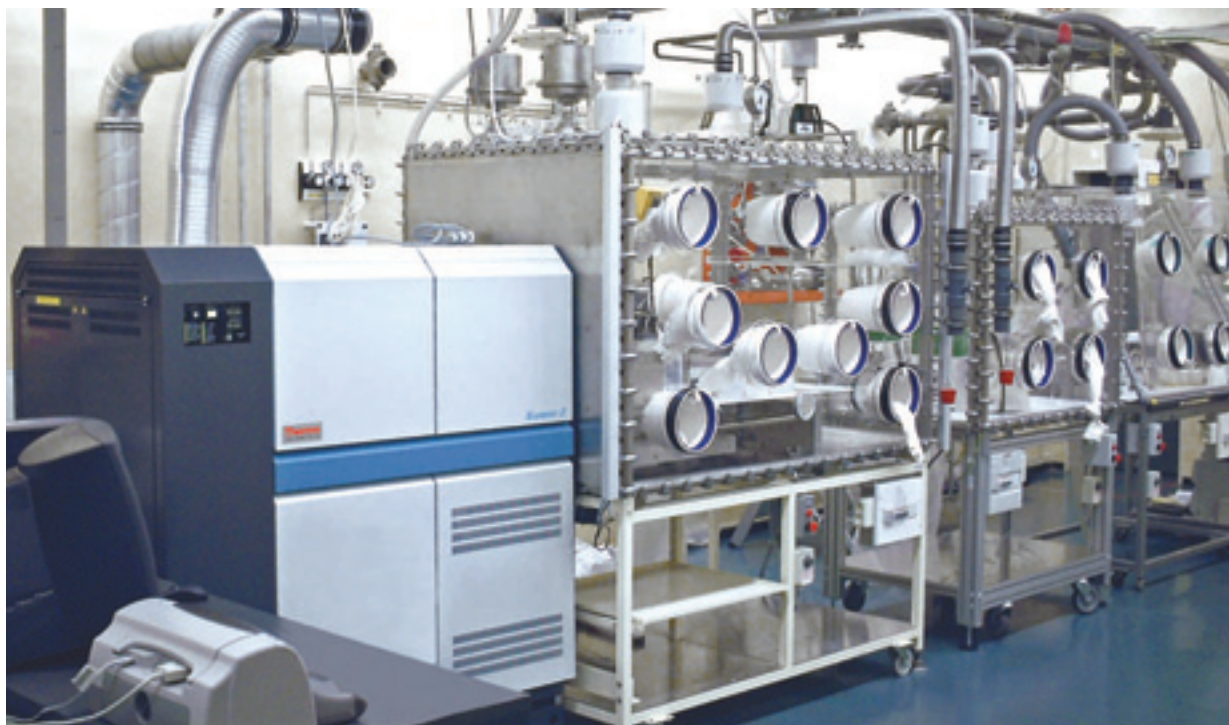
Figure 1: Thermo Scientific ELEMENT 2 adapted to a customer defined glovebox configuration.
