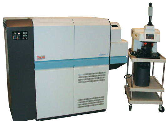
Figure 3: Thermo Scientific ELEMENT 2 with New Wave UP213 laser system.
