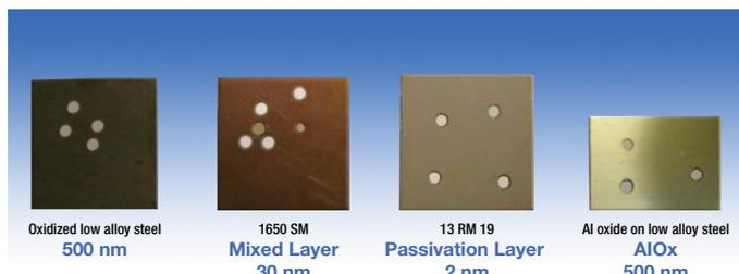
Figure 1. Iron based substrates with a variety of layer chemical compositions and thicknesses.
